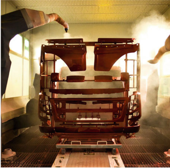
Fig. 3 Robotized spray painting of a Volvo truck cab using electrostatic rotary bells. Photo copyright: AB Volvo
