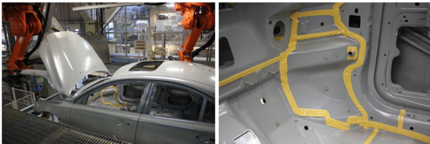
Fig. 2 A robot cell at Volvo Cars with two sealing robots applying material to the car body ( left ). Examples of interior sealing beads in the front passenger seat area applied by a flat bead sealing nozzle ( right ). Photos copyright: Volvo Cars
