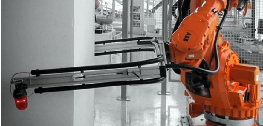
Fig. 1 Robotic Hot Wire cutting in Odense, Denmark
