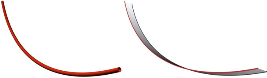
Fig. 8 Left : A cylindrical rod can cut in any direction that is close to perpendicular to the tangent of the curve. Right : A flat (ribbon) blade design (with its hot edge indicated in red) moves well only in the directions given by the flat extension of the blade past the hot edge itself
