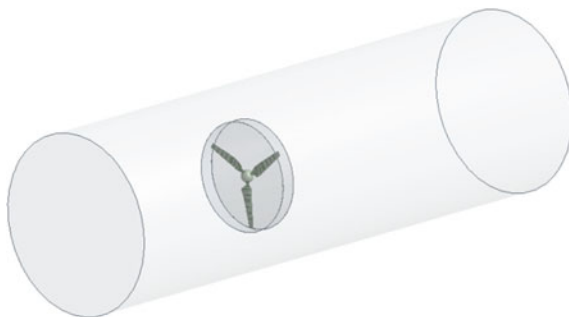
Fig. 2 CAD 3D calculation model of turbine with external finite area
