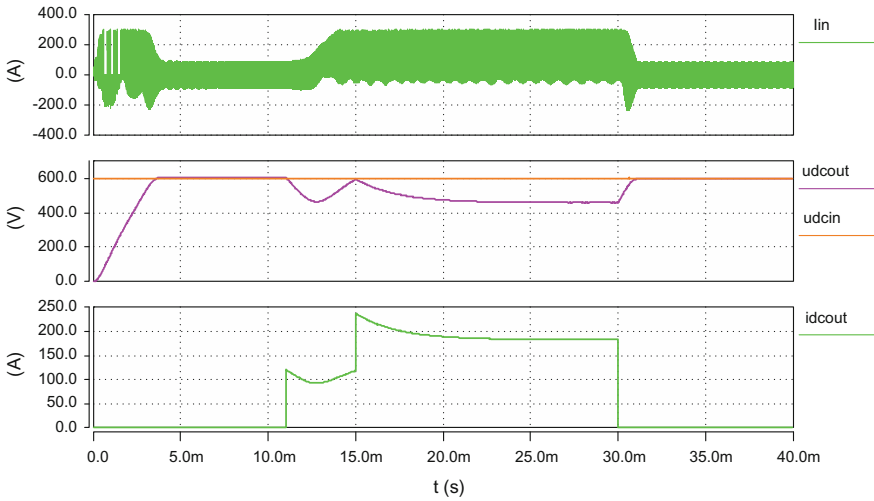
Fig. 11 ICET system response for load jumps
