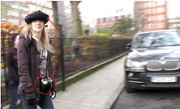
Fig. 2 Setting for real-life mapping of the prefrontal cortex activity by a wearable fNIRS system equipped with 22 channels (WOT-220, Hitachi High-Technologies Corporation, Japan). The flexible probe unit covers the head in correspondence of the underlying dorsolateral and the rostral prefrontal cortex. The processing unit is worn on the waist. Photo courtesy of Dr. Pinti (University College London). For details of the study (Pinti et al. 2015)
