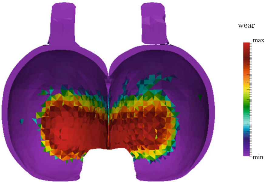
Fig. 2.11 Damage pattern with the Bitter model
