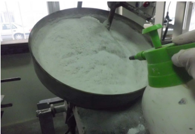
Fig. 1. Coating of expanded perlite surface with acid/silicate treatment in pellet machine
