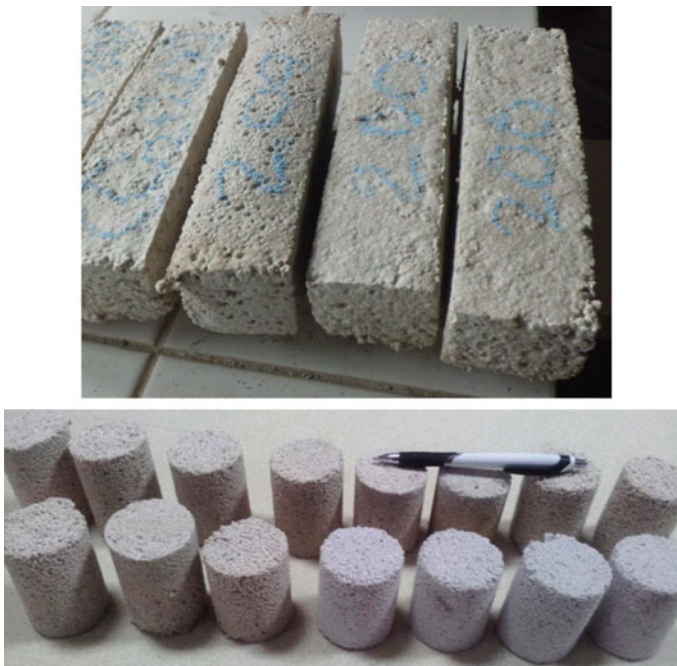
Fig. 5. The produced test specimens (40 × 40 × 160) mm prisms (top), and 50 mm diameter cylinders (bottom)
