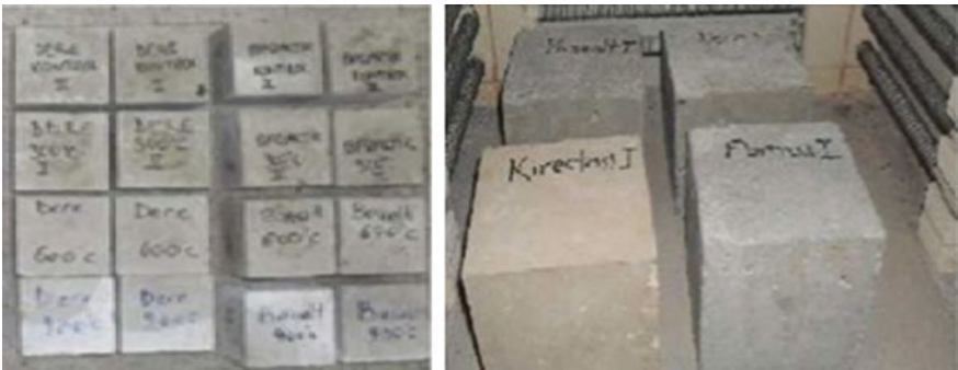
Fig. 2. The samples produced 10 \times 10 \times 10 cm and 15 \times 15 \times 15 cm in size
