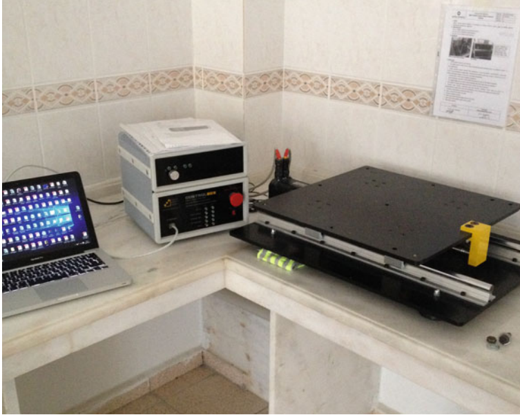
Fig. 3. Shaking table test device
