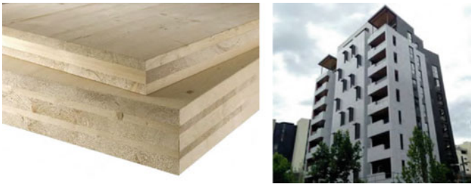
Fig. 5. Typical CLT Panels (left), Forte 10 storey residential CLT building in Melbourne (right)
