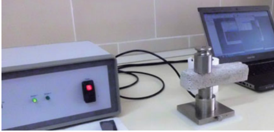
Fig. 6. Determination of \lambda values of samples (C-THERM device)
