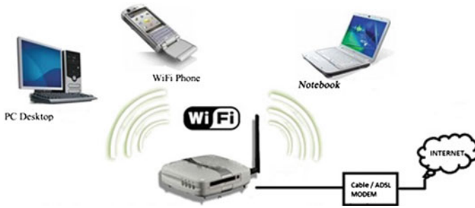
Fig. 1 Different WiFi client/station connections
