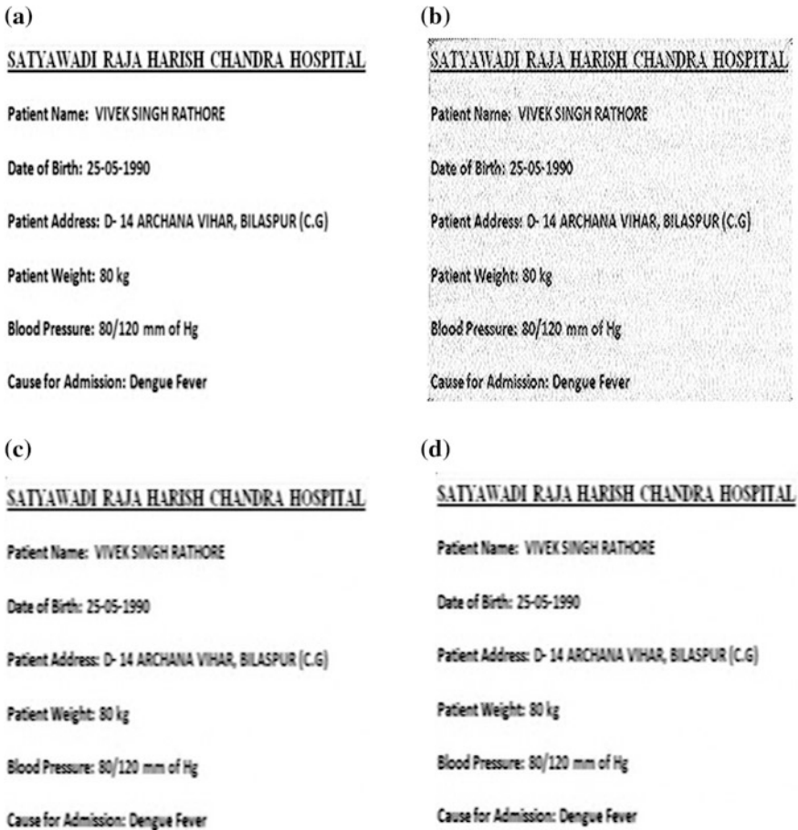
Fig. 6 a EPR as watermark image, and b–d recovered watermark image with gain factors 0.01, 1.0 and 5.0 for Fig. 5b–d respectively
