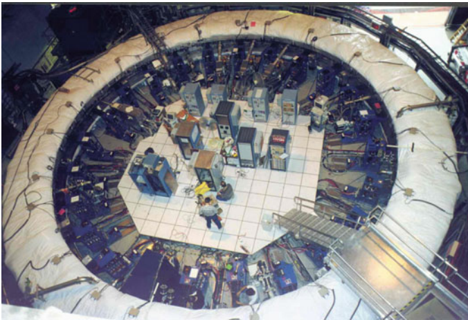
Fig. 6.2 The Brookhaven National Laboratory muon storage ring. The ring has a radius of 7.112 m, the aperture of the beam pipe is 90 mm, the field is 1.45 T and the momentum of the muon is p_\mu = 3.094 \text{ GeV}/c . Picture taken from the Muon g - 2 Collaboration Web Page http://www.g-2.bnl.gov/ (Courtesy of Brookhaven National Laboratory)
