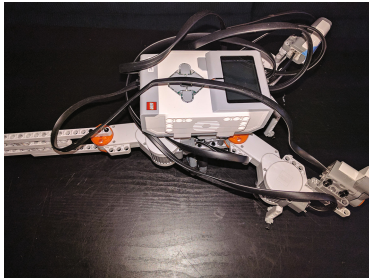
Fig. 3. Physical robot made out of Legos. Can represent the \mathcal{M} or \mathcal{NM} robot by fixing/freeing motors.
