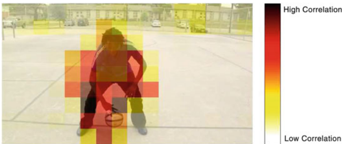
Fig. 9.3 CCA illustration: heat map showing correlation between video image regions and audio. Black squares indicate highest correlation
