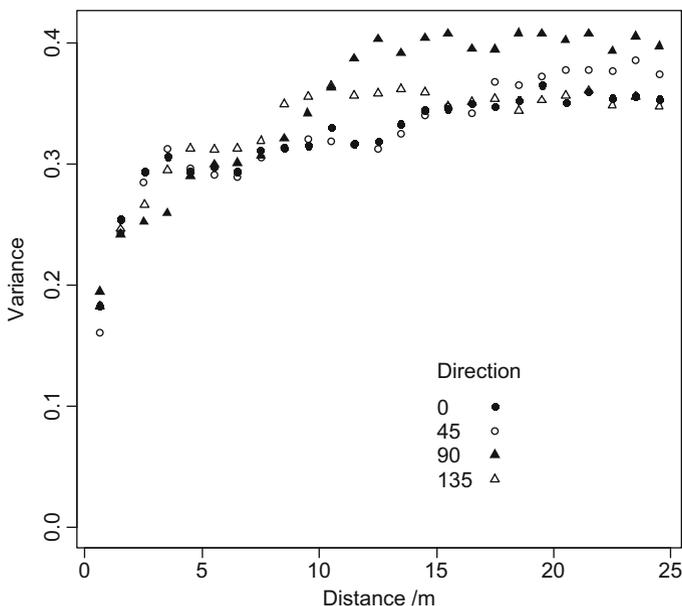
Fig. 10.7 Directional empirical variograms of log copper content
