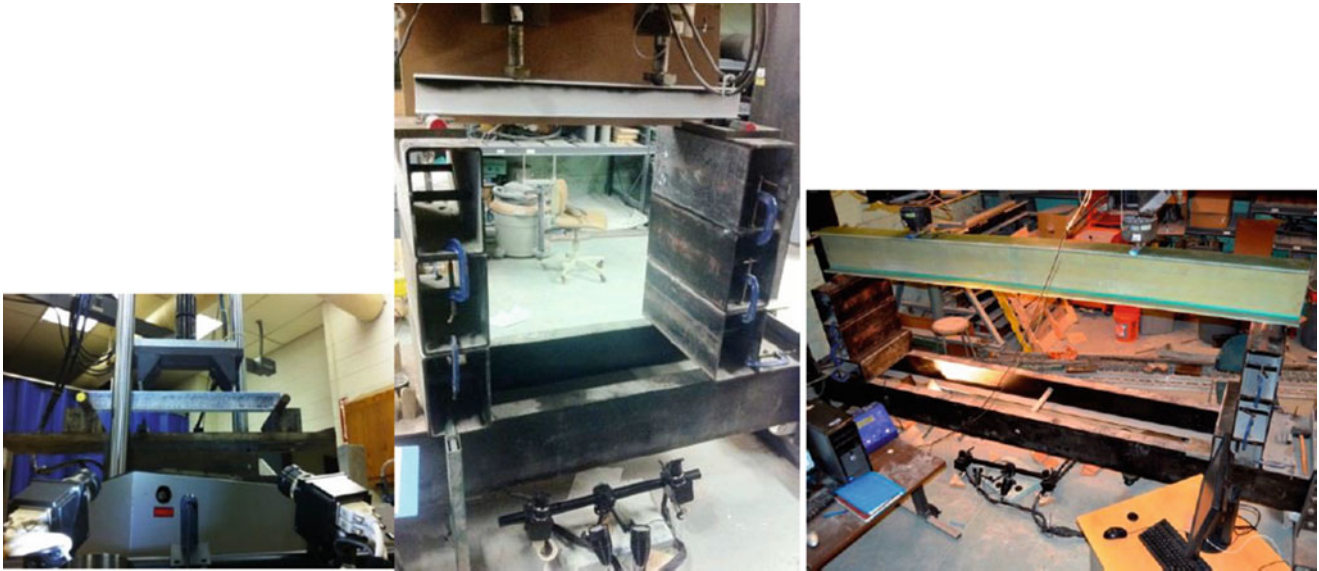
Fig. 7.3 Quasi-static flexural bending test setup for small beams ( left ), medium beams ( middle ) and large beams ( right )
