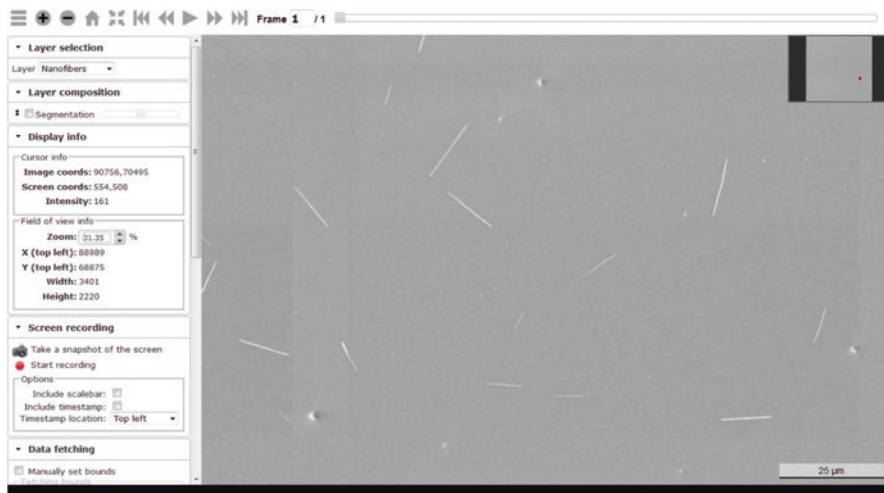
Fig. 1.3 Images of aerosolized carbon nanotubes collected on a Si wafer imaged over 2360 overlapping FOVs. The data is available online ( https://isg.nist.gov/deepzoomweb/data/materialparticlesdistribution )
