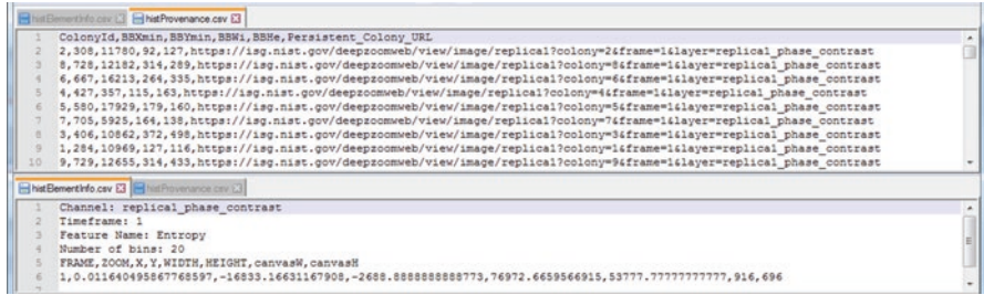
Fig. 4.24 Two additional files saved from the web statistical modeling tool that contain all pyramid coordinates and hyperlinks of thumbnails (top) and all information about the histogram parameters
