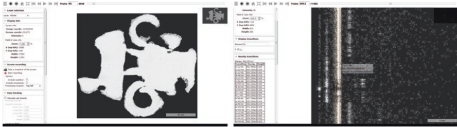
Fig. 5.27 A spatial view of a historical artifact ( https://isg.nist.gov/deepzoomweb/data/materiale-energylevels ) imaged using an electron microscope (left) and its re-projected spectral view [y, \lambda] for one of the x -cross sections (right)
