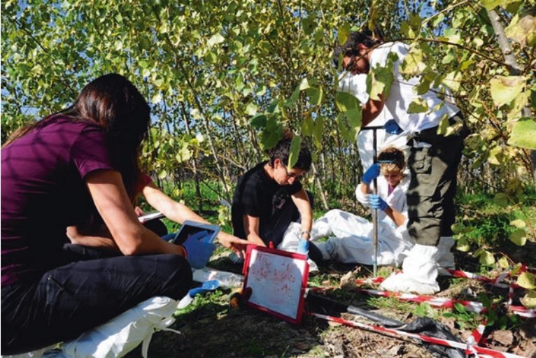
Fig. 18.3 Soil sampling from a PCB historically contaminated area, located in Southern Italy and planted with poplar (Ancona et al. 2017)
