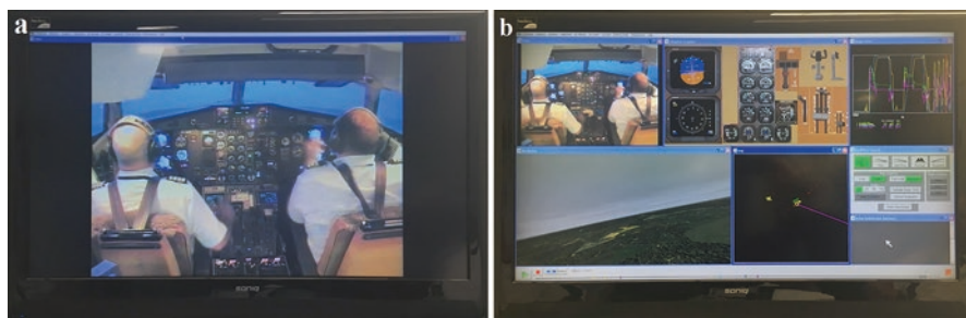
Fig. 8.3 Two possible views available to a flight examiner with the “debriefing tool”. (a) Full screen video/audio recording of the flight deck: This view is typically used by the flight examiner to demonstrate pilot interaction and specific behaviours such as decision-making and management. (b) More comprehensive view: This view provides, in addition to the flight deck, an integration of recorded information on flight, engine, and system instruments that are used for pilots to demonstrate flying manoeuvres during the simulator session. It enables the status of instruments during an emergency exercise to be replayed
