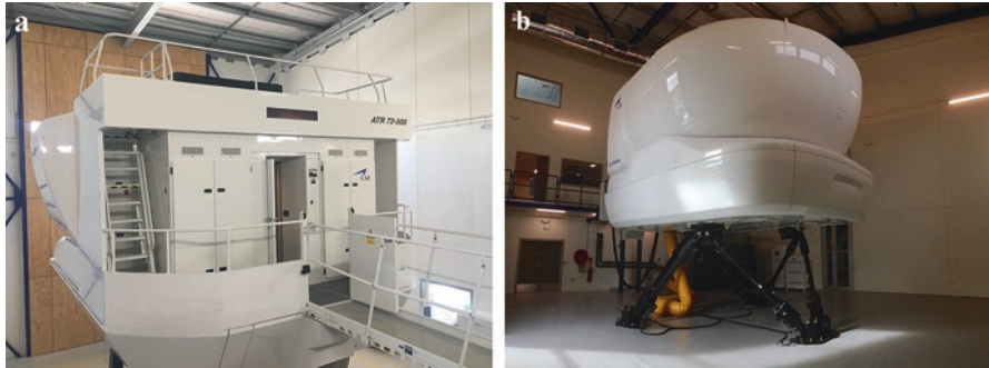
Fig. 8.1 (a) The modern flight simulator is a large device that houses an exact mock-up of the aircraft but also contains an advanced visual system that is wrapped around the front of the simulator. (b) The high-fidelity simulator is on jacks allowing true sensation of turbulence, acceleration, and deceleration to be transferred to the pilots
