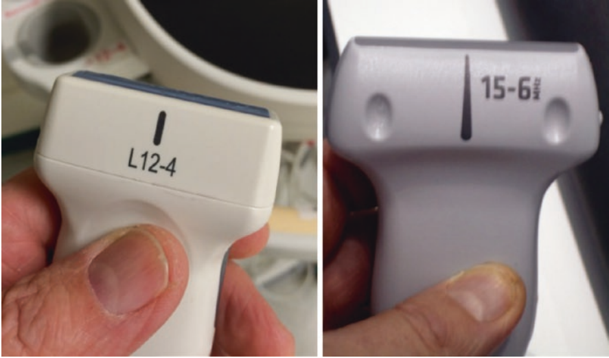
Fig. 13.54 Newer point-of-care US machines now have a midline mark etched on the short axis face of their linear array and curved array transducers. This improves your “map and mark” and free-hand procedure accuracy
