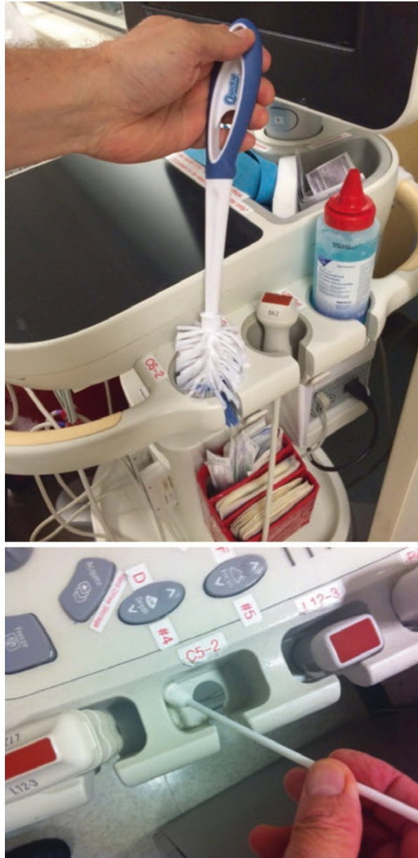
Fig. 13.12 A short bottle brush or GYN Q-tips work well for cleaning out dust and gel from transducer cup holders
