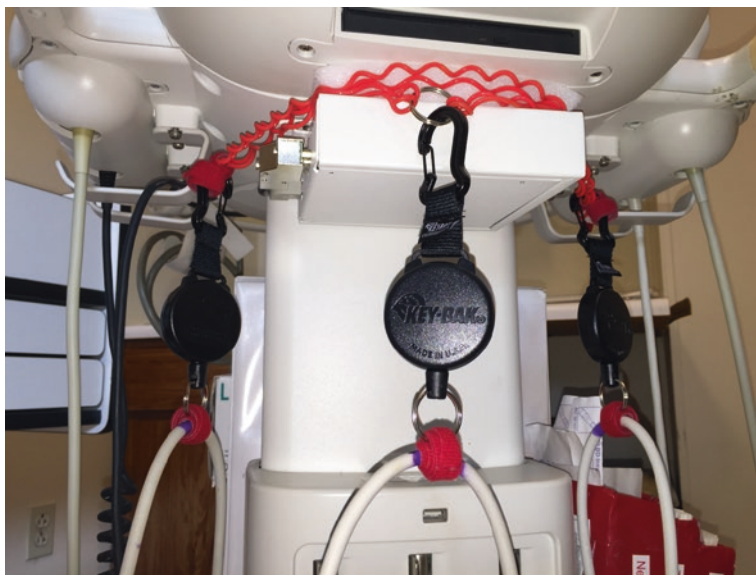
Fig. 13.37 Key fob bungee set up, same idea, key fobs used instead of extension springs
