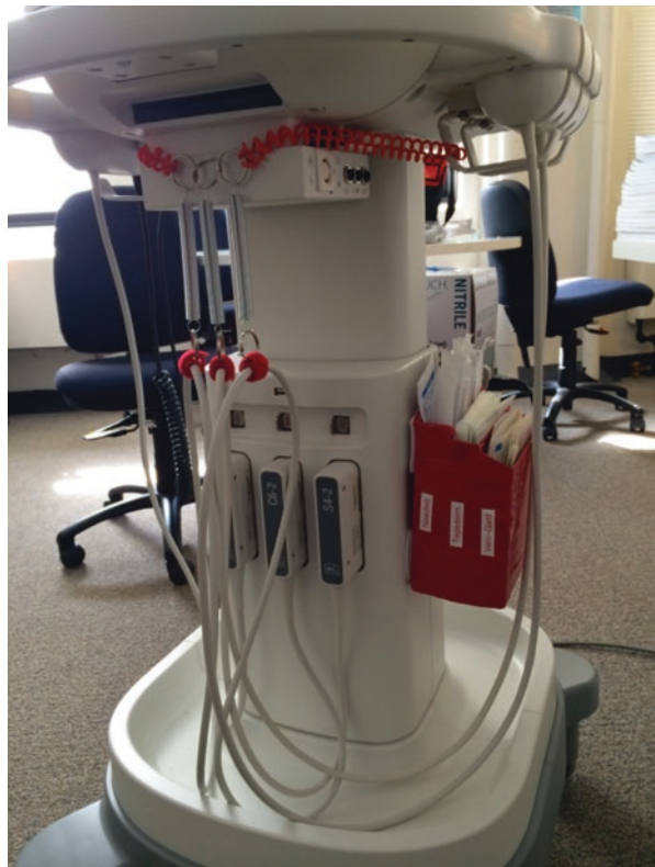
Fig. 13.48 Your new homemade supply organizer attached to the cart with industrial Velcro sticky-back tape
