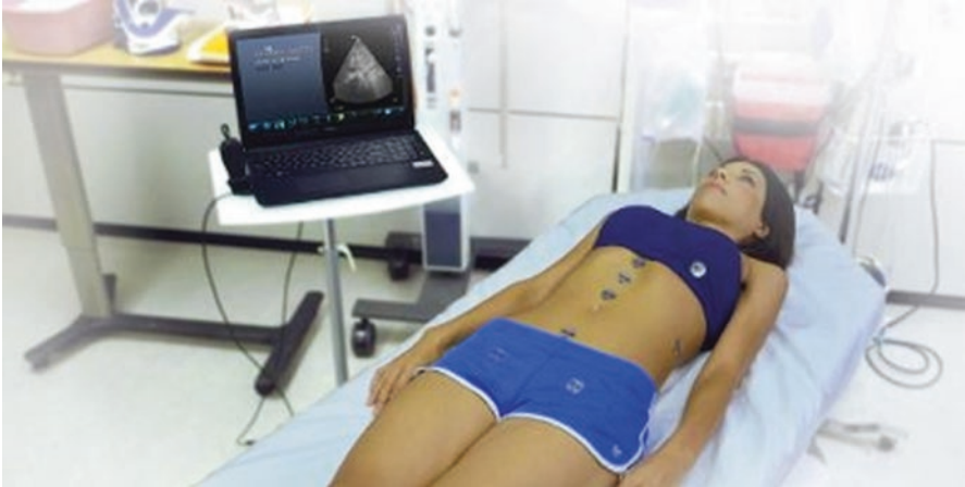
Fig. 11.5 The SonoSim® LiveScan (SonoSim, Santa Monica, CA) anatomic simulator uses simulated ultrasound equipment, real and simulated patient anatomy, and real-time dynamic scanning through the imaging data set which is localized to the proper anatomic location using ID tags placed on the model
