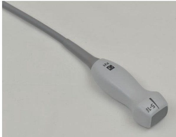
Fig. 12.23 Phased array transducer
