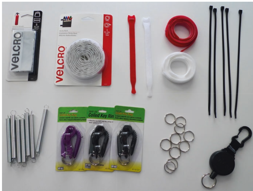
Fig. 13.30 Essential customizing supplies for new machines include: industrial and regular Velcro sticky-back tape, Velcro cable ties, plastic cable ties, piano wire extension springs, coiled key, metal key rings, and robust key fobs
