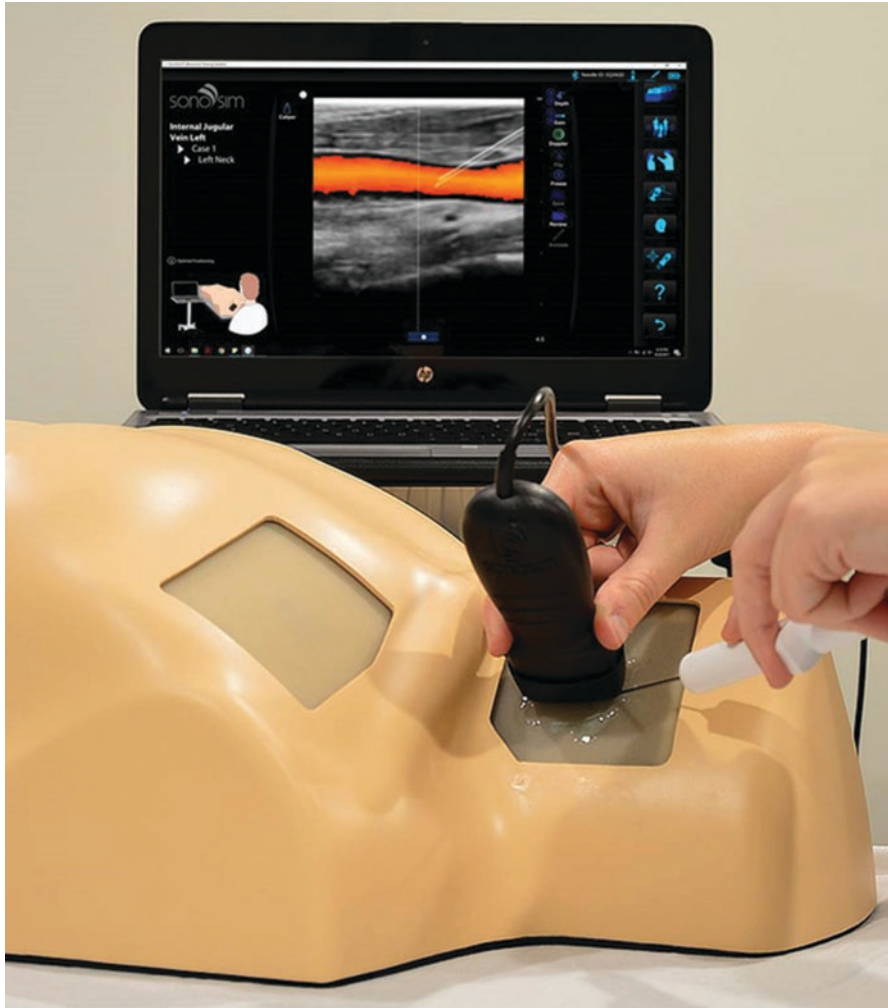
Fig. 11.4 Laerdal (Stavenger, Norway) Laerdal-SonoSim Procedure Trainer - first release includes a vascular access simulator using real patient anatomy that features color, power, and spectral Doppler tracings, automated real-time performance assessment, and virtual instruction. Anatomic Simulator: Live Model
