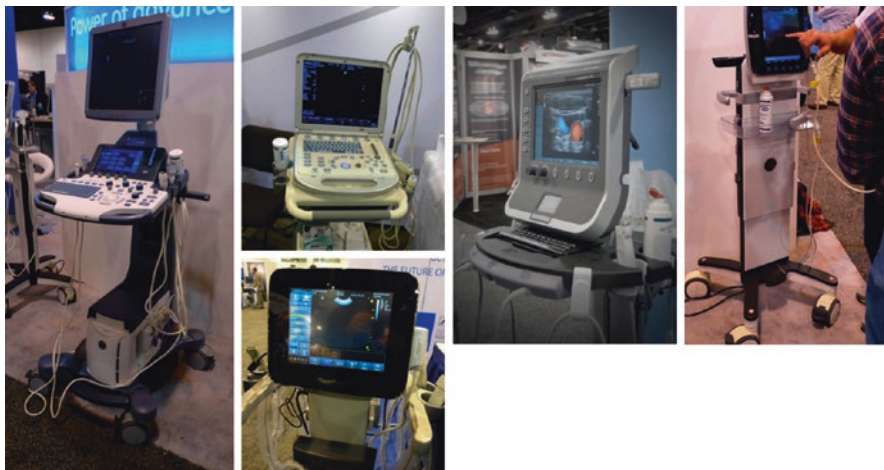
Fig. 13.6 Choosing your equipment: assess control surface layouts, user interfaces, and overall ease of use. Look at how transducer cords are managed, how easy the control surfaces are to clean, ease of cart mobility, are there locations for supplies that you will want on the cart?
