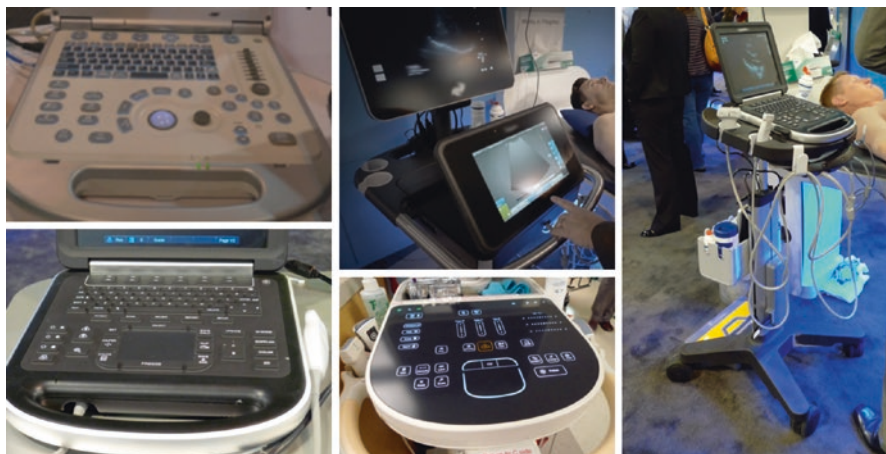
Fig. 13.5 Choosing your equipment: assess control surface layouts, user interfaces, and overall ease of use. Look at how transducer cords are managed, how easy the control surfaces are to clean, ease of cart mobility, are there locations for supplies that you will want on the cart?
