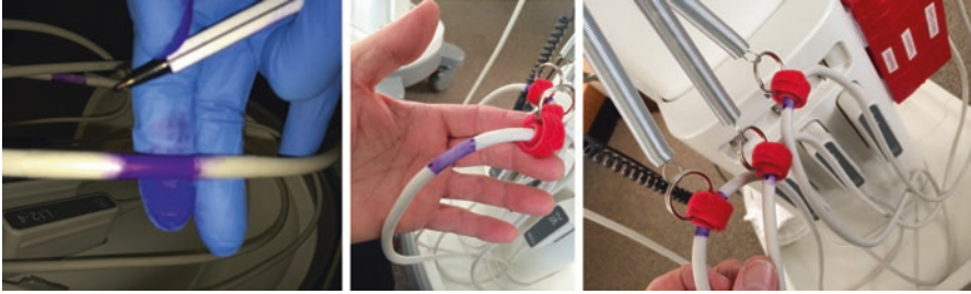
Fig. 13.38 Mark the sweet spot along the cord where the Velcro cable tie keeps the transducer cord off the floor. Tape off the area first, wear gloves, and remove tape when dry. The transducer cord can slide out from its usual attachment site if a longer length is needed for a procedure. Return the cable tie and cord bungee back to the easily visible “sweet spot” when done
