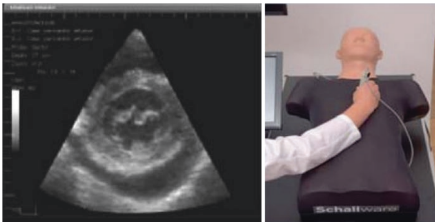
Fig. 11.13 The Schallware (Berlin, Germany) anatomic simulator uses simulated ultrasound equipment, real patient anatomy, and real-time dynamic scanning through the imaging data set
