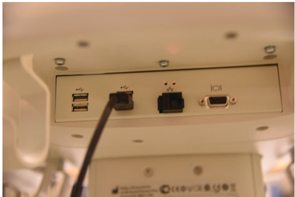
Fig. 12.11 Video input and output digital connections
