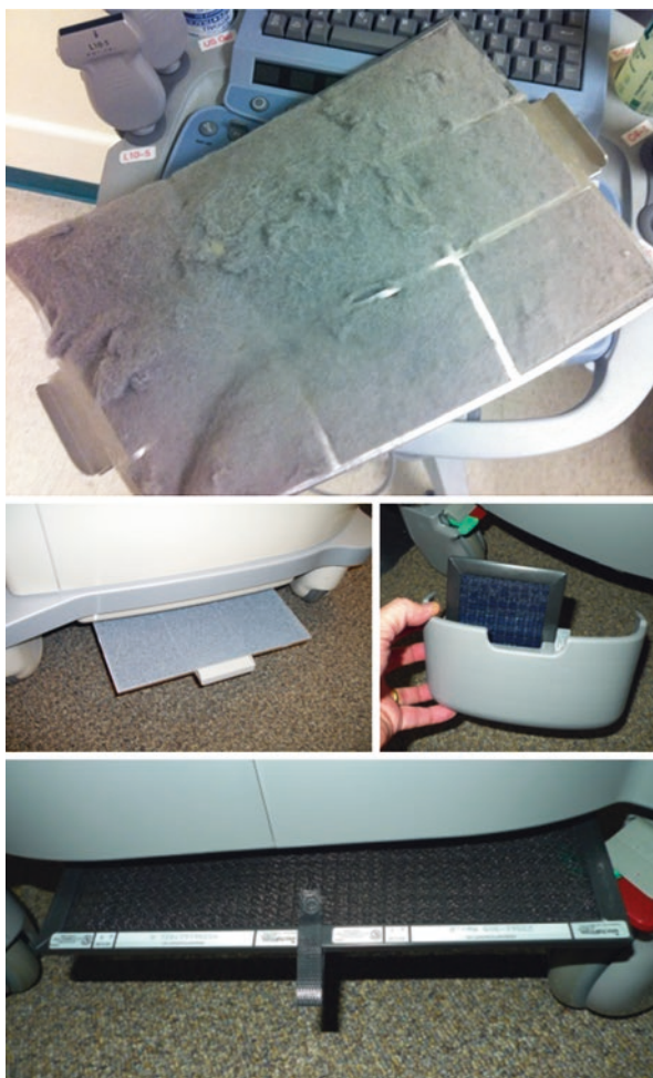
Fig. 13.23 The ER is a very dusty place. Onboard filters should be cleaned every several months to avoid overheated electronics. Once a year cleaning is inadequate
