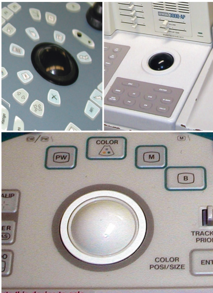
Fig. 13.22 Trackballs need periodic cleaning to remove ultrasound gel that can impede smooth trackball function
