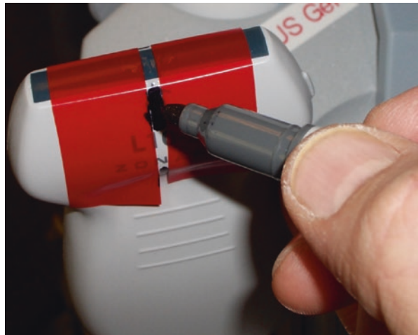
Fig. 13.54 Newer point-of-care US machines now have a midline mark etched on the short axis face of their linear array and curved array transducers. This improves your “map and mark” and free-hand procedure accuracy
