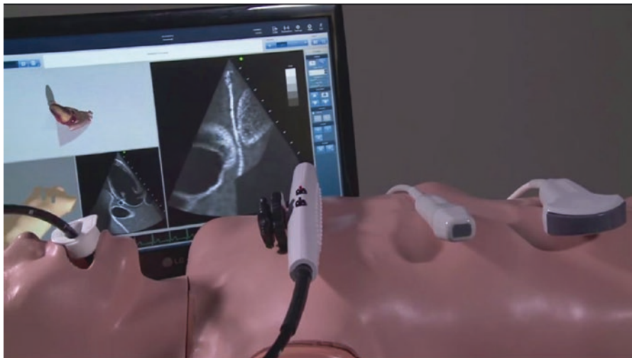
Fig. 11.9 The Vimedix system (CAE Healthcare) uses simulated ultrasound equipment, simulated patient anatomy, and real-time dynamic scanning through the imaging data set
