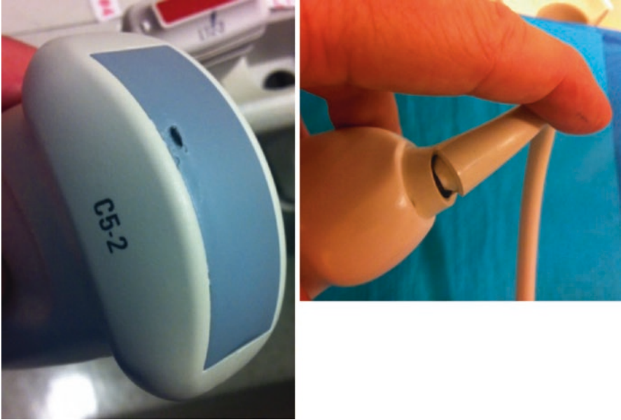
Fig. 13.13 Transducers with visible defects such as these will need to be replaced
