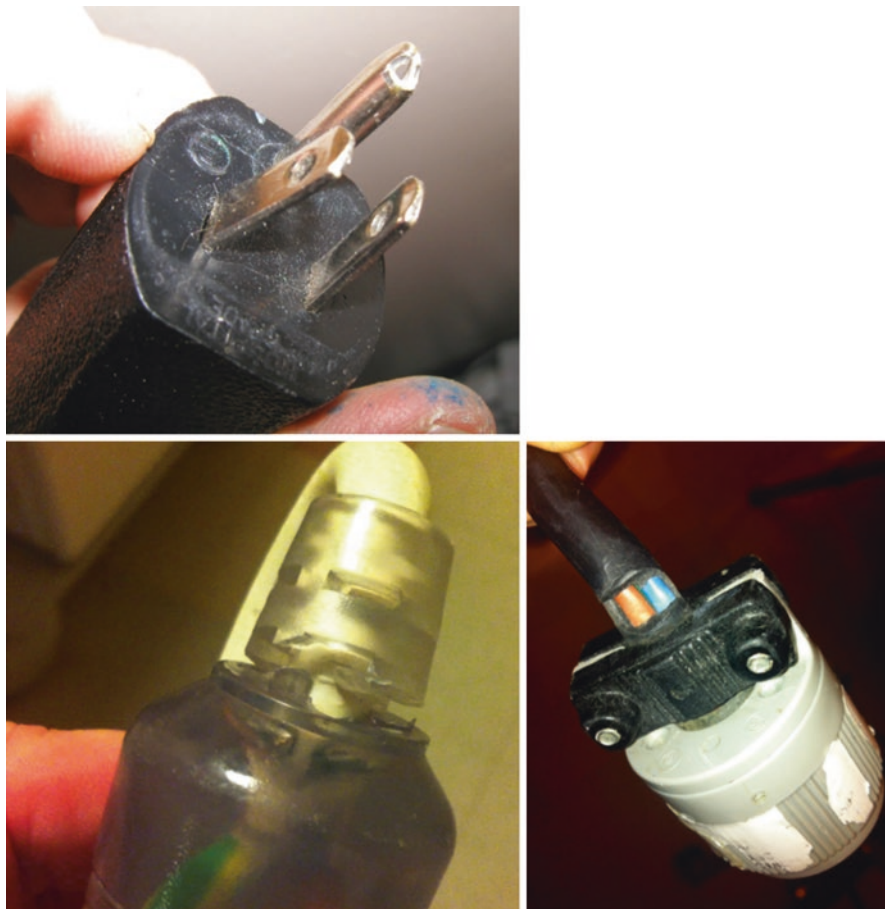
Fig. 13.28 Power cord plug end woes: bent pins, a cracked housing, exposed wires: all bad, time for replacement
