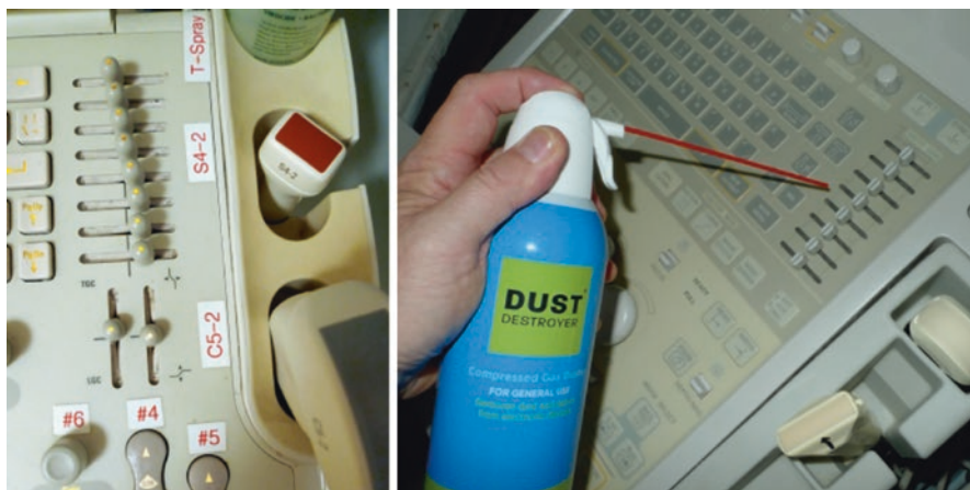
Fig. 13.17 A can of compressed air will help clean out dusty TGC buttons on older machines
