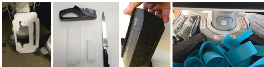
Fig. 13.46 Save the hard packing foam that arrives with a new machine. You can easily cut it into custom dividers for your storage areas. Use Velcro sticky-back tape to hold the dividers in place
