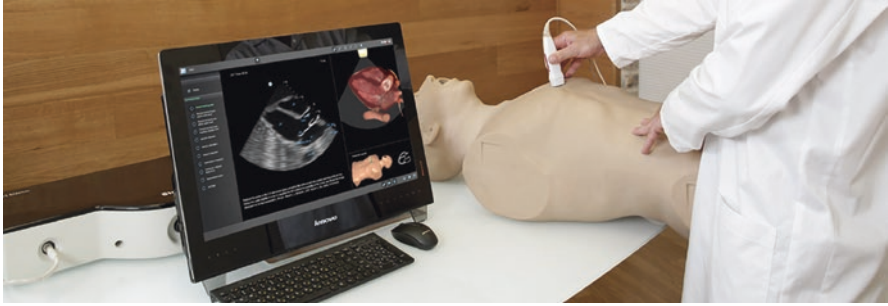
Fig. 11.10 The U/S Mentor (Simbionix, Airport City, Israel) anatomic simulator uses simulated ultrasound equipment, simulated patient anatomy, and real-time dynamic scanning through the imaging data set
