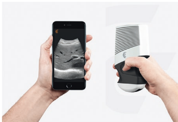
Fig. 12.30 Smart phone controlled portable ultrasound
