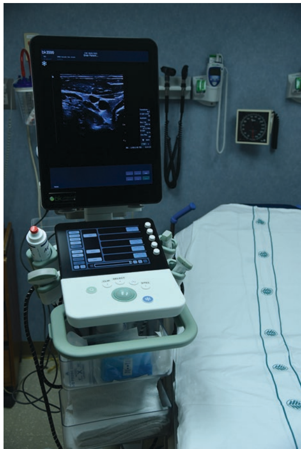
Fig. 12.14 Touchscreen and hard controls
