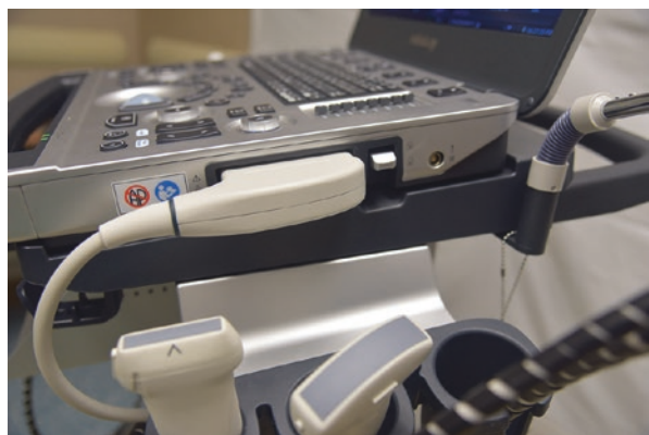
Fig. 12.27 Probe connection into laptop
