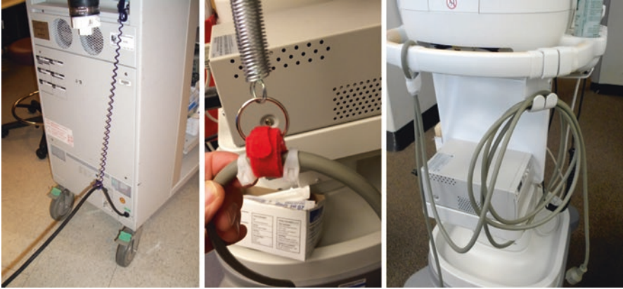
Fig. 13.41 Three power cord tethering solutions: use a coiled key ring bungee, or a more robust extension spring, or tether the power cord to the back handle of the cart if this option is available. See Fig. 13.36c for the custom power cord bungee option
