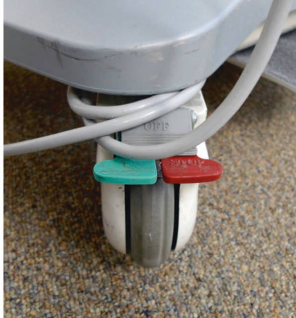
Fig. 13.31 A transducer cord wrapped around a cart caster wheel; guaranteed agitation
