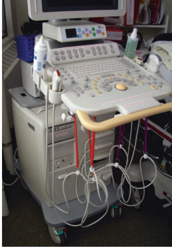
Fig. 13.35 A four-transducer ultrasound machine with cord bungees in place; note that the cords never touch the floor
