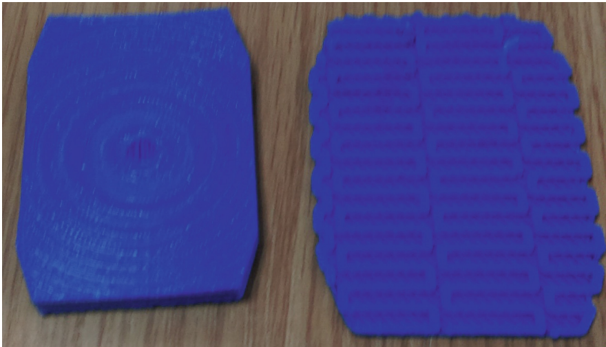
Fig. 6. Printed camera base (left) on MAKERBOT printer with built support (right).
