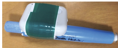
Fig. 2. A chalk holder with an acceleration sensor (AccelChalk)
