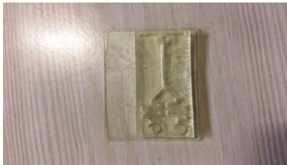
Fig. 6.3 3D printed output of the microviscometer
