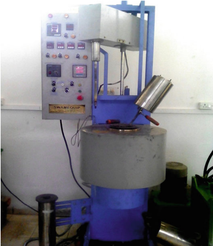
Fig. 29.1 Stir casting furnace
