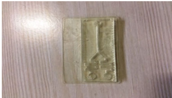
Fig. 6.3 3D printed output of the microviscometer
