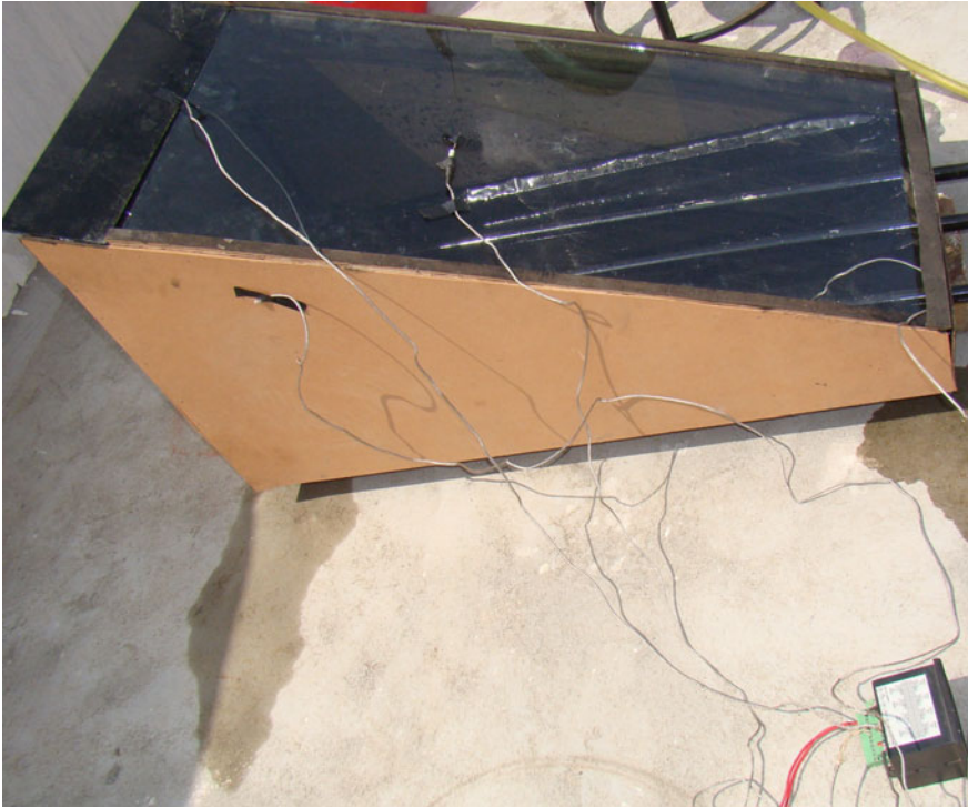
Fig. 17.1 Solar still with thermocouple display
