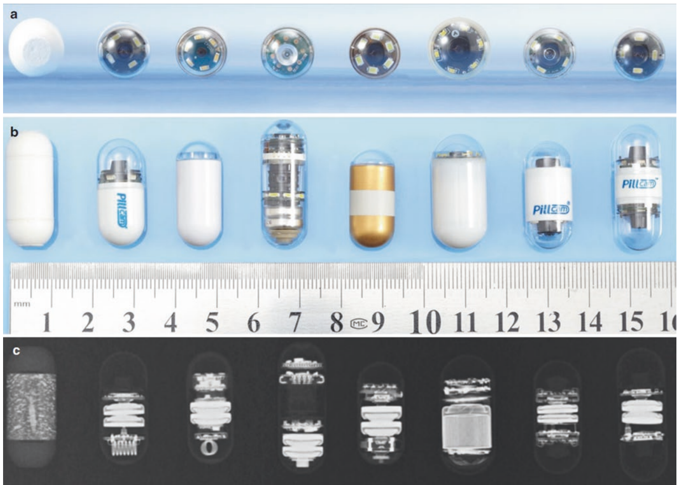
Fig. 18.1 Comparison of different video capsules. Front view (a) and top view (b) of the capsules, with corresponding X-ray image (c). Left to right: Agile patency capsule, PillCam SB2, EndoCapsule, CapsoCam, MiroCam, OMOM capsule, PillCam ES02, PillCam Colon 2. Adapted from Kurniawan and Keuchel. [4,5] With permission of Springer Nature.
