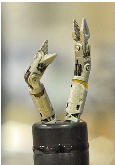
Fig. 41.9 Twin 7 DOF arms on Endomaster's MASTER robot (Reproduced with permission. Source: [ www.endomastermedical.com ])
