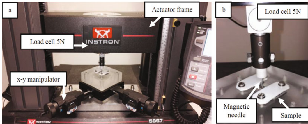
Fig. 1.3 Experimental setup for the magnetic balance method: (a) sample holder and the x-y manipulators, and (b) a close-up of the magnetic needle
