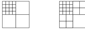
Fig. 2. 2:1 balance status for a 2D quadtree mesh: unbalanced (left) and face balanced (right).
