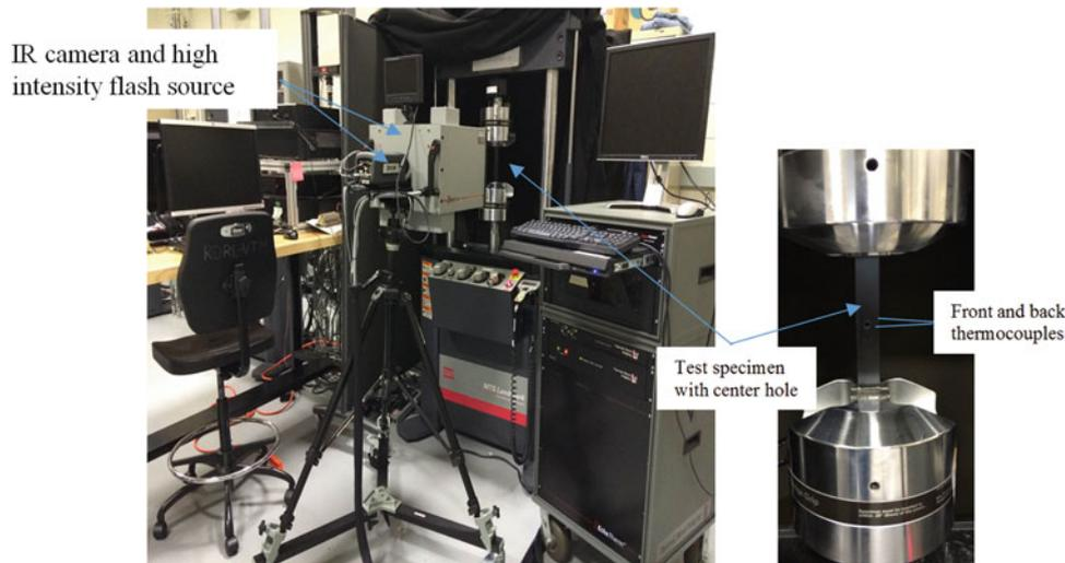
**Fig. 15.2** Experimental setup showing the pulsed thermography. The test sample is a rectangular carbon-epoxy laminate with a centre (fastener) hole. Two thermocouples are attached at the front and back near the centre hole in the mode-I direction. Surface temperatures are measured after the application of the high intensity flash at the front of the specimen
