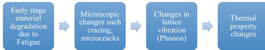
**Fig. 15.1** Changes in microscopic material state (or configuration) due to stress concentration, shear localization, adiabatic shear bands, crazing, dislocation that typically appear in the early stage of fatigue damage, may be correlated to changes in the thermophysical properties
