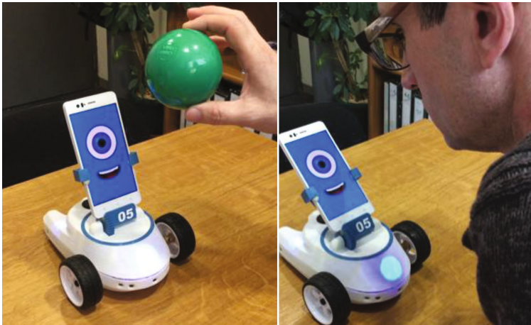
Fig. 6. The user showing a green ball that represents “food” (left) and his face, which makes Robobo move backwards (right)
