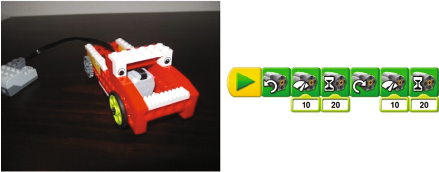
Fig. 1. Robotic model, which was built according to instructions (on left) and pupils' own program to control it (on right).
