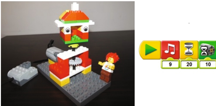
Fig. 2. Robotic model, which was built according to instructions (on left) and program from worksheet to control it (on right).
