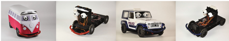
Fig. 3. Two DIY mobile social robots created using the OTO platform.
