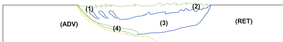
Fig. 7.6 Distinct regions in weld nugget for the case of friction stir welded dissimilar titanium alloys
