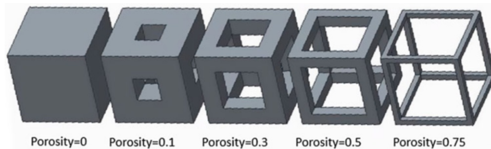
Fig. 8.3 Schematic of unit cells with different porosities
