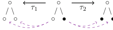
Fig. 2. Using orbits to deduce origins. We represent the orbits with colours: \circ are nodes of orbit 0, \bullet are nodes of orbit 1. We apply two transformations \tau_1 and \tau_2 on an input tree (here in the middle): \tau_1 replaces its right leaf by a copy of the left one, while \tau_2 replaces its left leaf by a copy of the right one. Without the orbits, these two transformations would look identical. However, as seen above, the orbits allow a distinction between \tau_1 and \tau_2 for some input tree.
