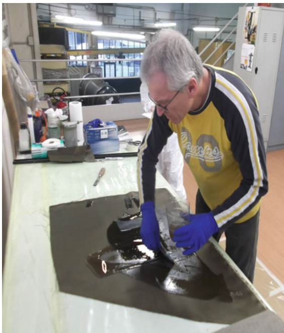
Fig. 4 The dry fabric has been impregnated by pouring the resin on top and distributing it along the entire surface, using a spatula
