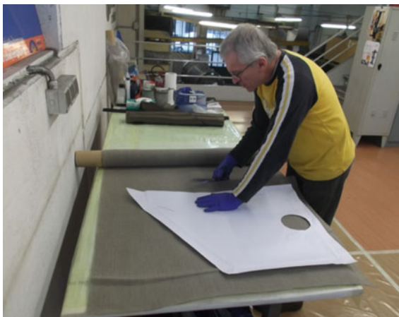
Fig. 2 The edges of the fabrics have been trimmed from the wires coming out
