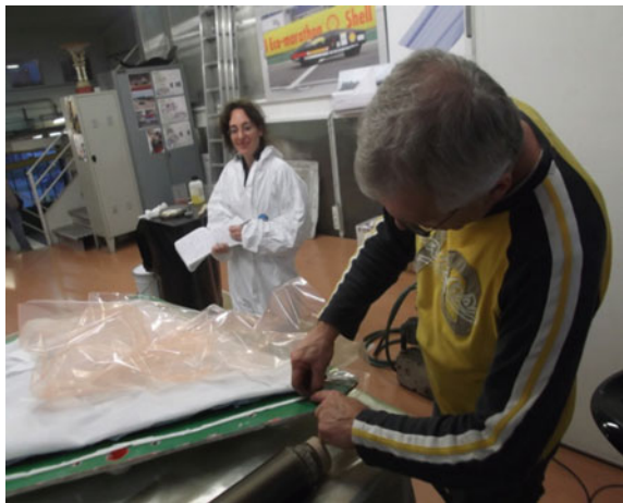
Fig. 13 The vacuum bag has been fixed to the mould, all along its perimeter, by means of a double-sided high thickness tape
