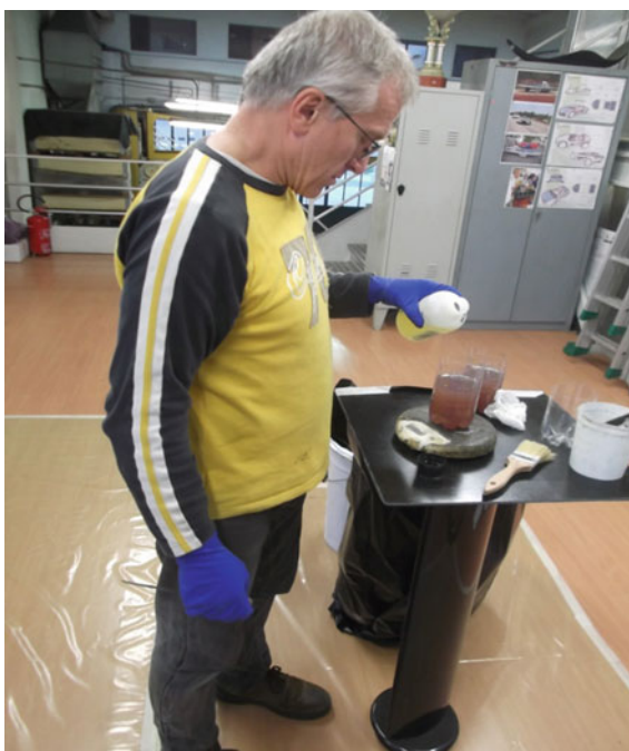
Fig. 3 The resin has been prepared by mixing it with catalys in exact proportions
