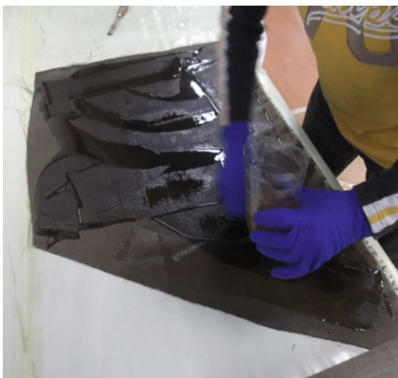
Fig. 5 The fabric made of flax has been placed on the previous one, flattening it
