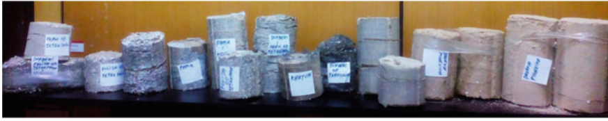
Fig. 2 Samples of 13 different composite materials completely made of waste materials
