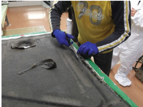
Fig. 9 The hole has been reinforced with the remaining fabric scraps
