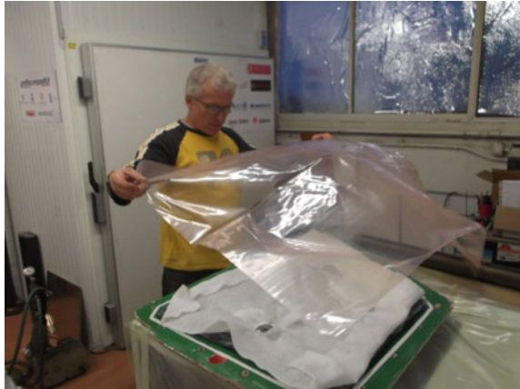
Fig. 12 The vacuum bag has been applied with extreme care to avoid damage in positioning
