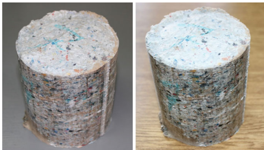
Fig. 5 Sample C7 prior to ( left ) and after ( right ) the compressive loading test
