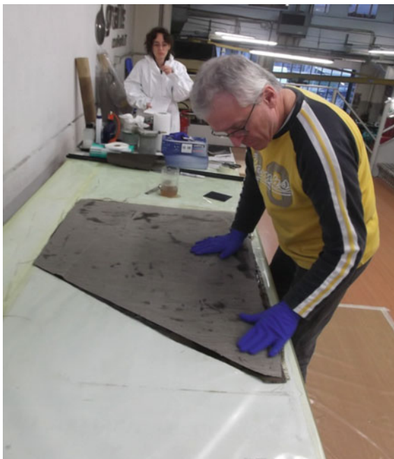
Fig. 6 The other resin has been poured and spread until complete impregnation
