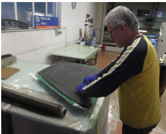
Fig. 7 Extreme care has been paid to the fastening of the fabric that, once stretched, has to be retained in position to prevent shifting or folds
