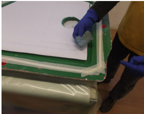
Fig. 1 A model in cardboard has been realized, and trimmed according to the geometry
