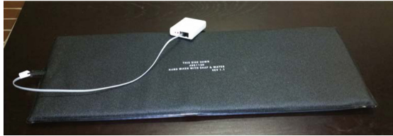
Fig. 2. Self-calibrating mat sensor, for under-the-mattress positioning.
