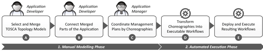
Fig. 3. Steps of the method to systematically reuse TOSCA-based (i) application topologies and (ii) their corresponding management plans.
