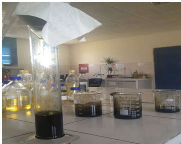
Fig. 6 Distilled medical waste plastic fuel samples
