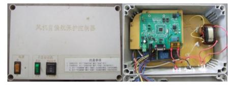
Fig. 17 Furling controller of the wind turbine prototype
