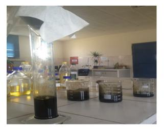
**Fig. 6** Distilled medical waste plastic fuel samples
