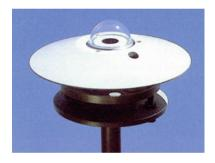
Fig. 2 The solar integrator used
