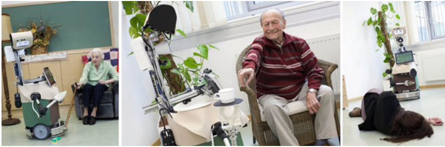
Fig. 5.13 The Hobbbit robot in three robot tasks: bring an object, pick-up an object from the floor, and detect an emergency situation [52]
