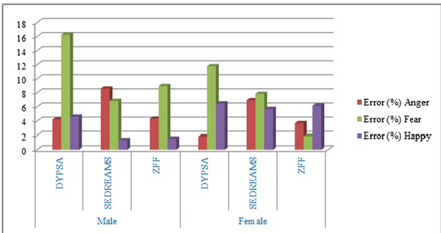
Fig. 2. Comparison of various GCI algorithms based on percentage error. The values are calculated based on median of anger, fear and happy emotions for both male and female speakers
