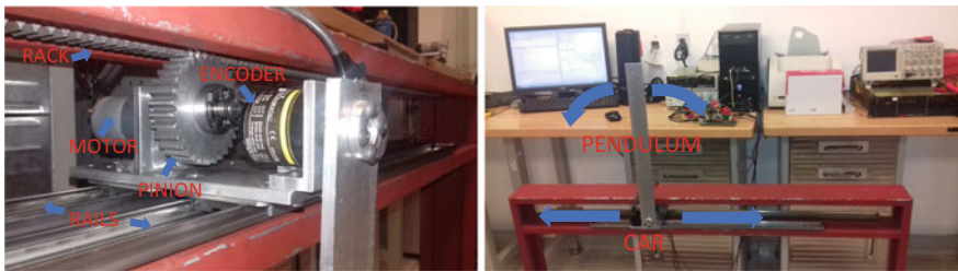
Fig. 4.8 Experimental platform of the inverted pendulum on a car system
