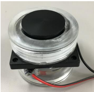
Fig. 6. EL transducer prototype
