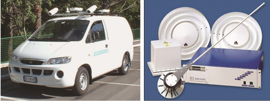
Fig. 2. The MMS of the GeoSNav Lab, University of Trieste, and the Applanix Corporation POS LV ® system components mounted on board the vehicle.
