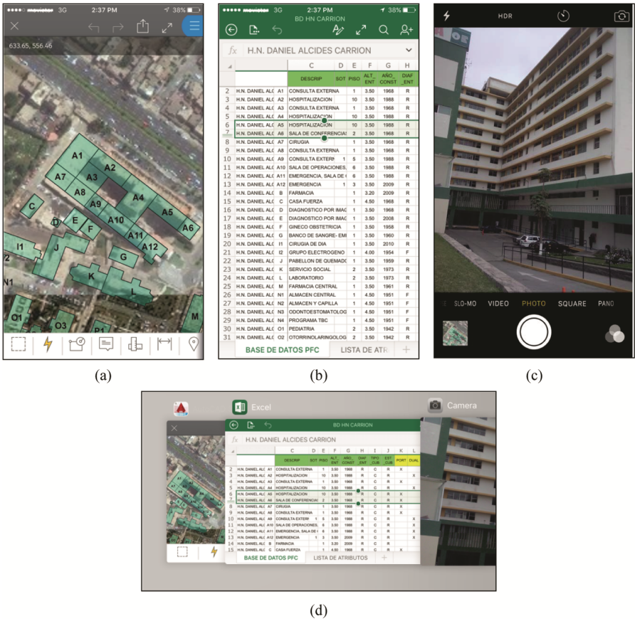
Fig. 3. Field data collection using mobile devices: (a) georeferencing, (b) data collection form, (c) photographing, (d) multitasking environment
