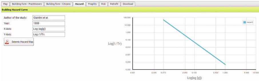
Fig. 16. Tab Hazard – Hazard curve for soil “C”.
