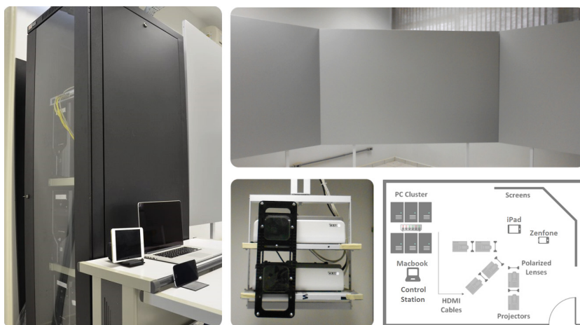
Fig. 3. Devices used with Dimmol and their arrangement. Each of MiniCAVE's three screens has area of 3.75 \text{ m}^2 ( 2.5 \text{ m} \times 1.5 \text{ m} ). Adapted from [24].
