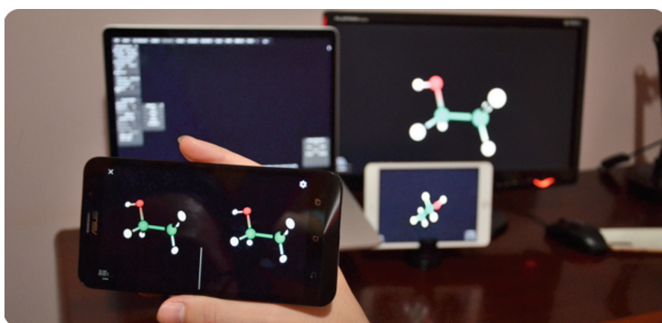
Fig. 6. Configuration using Macbook (master), Windows PC (slave), iPad (slave, free visualization), Android phone (slave, Google VR).
