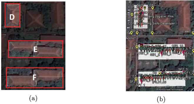
Fig. 3. (a) The picture of the buildings captured from above using Google Earth. (b) The overlaid of multi-two dimensional spaces model with the points of rooms, corridors, and stairs.
