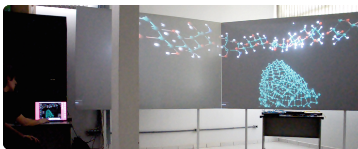
Fig. 4. Configuration using Macbook (master) and MiniCAVE cluster (slaves).
