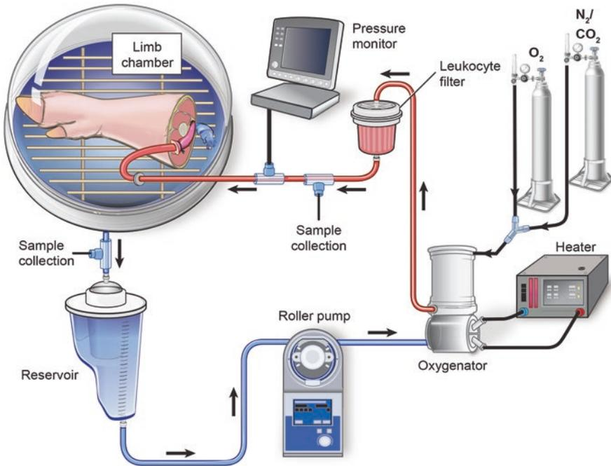
**Fig. 2.4** Schematic of a normothermic perfusion system for the limb. (Reprinted with permission, Cleveland Clinic Center for Medical Art & Photography © 2014-2016. All Rights Reserved)
