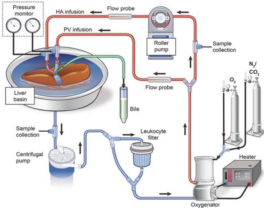
**Fig. 2.2** Schematic of a normothermic perfusion system for the liver. (Reprinted with permission, Cleveland Clinic Center for Medical Art & Photography © 2014-2016. All Rights Reserved)
