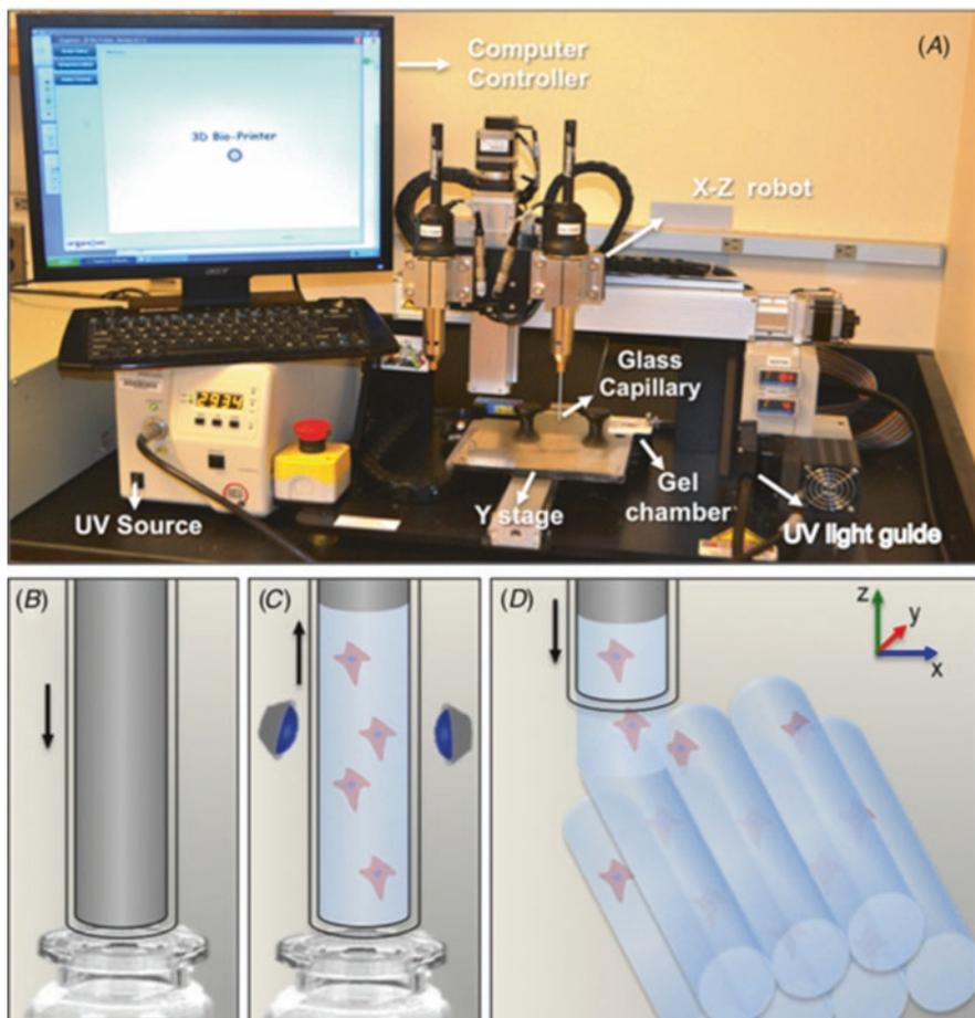
**Fig. 11.6** (a) Photograph of an Organovo Bioprinter setup, (b) metallic cylinder immersed in a vial containing cells and a hydrogel precursor. (c) Upward aspiration of the cell-laden hydrogel. (d) Precise printing of cell-laden hydrogel fibers [3]
