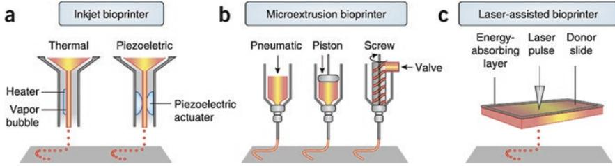
**Fig. 11.2** Comparison of material deposition between inkjet, micro-extrusion, and laser-assisted bioprinters (Reprint permission by Murphy and Atala [22]. Copyright (2016))
