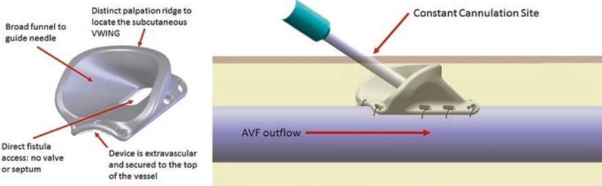
**Fig. 4.9** VWING device (From the manufacturer, Vital Access, and Galt et al. [43], used with permission)
