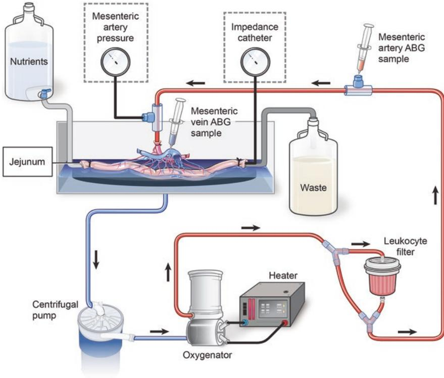
**Fig. 2.3** Schematic of a normothermic perfusion system for the intestine. (Reprinted with permission, Cleveland Clinic Center for Medical Art & Photography © 2014–2016. All Rights Reserved)
