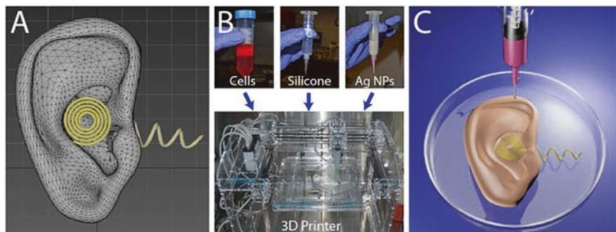
**Fig. 11.3** (a) Computer software used to design the bionic ear, (b) material mixtures used in 3D printer, (c) printing of a bionic ear (Reprinted with permission from Mannoor et al. [16]. Copyright (2016) American Chemical Society)
