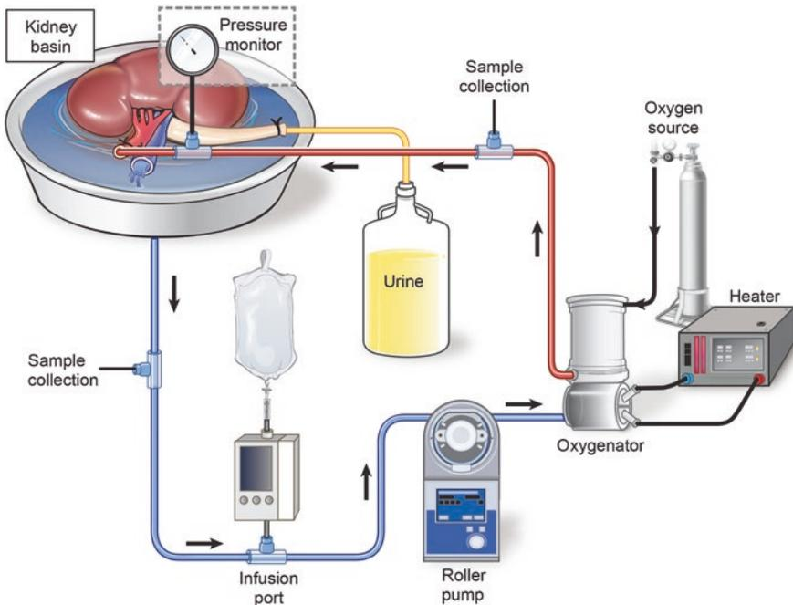
**Fig. 2.1** Schematic of a normothermic perfusion system for the kidney. (Reprinted with permission, Cleveland Clinic Center for Medical Art & Photography © 2014-2016. All Rights Reserved)
