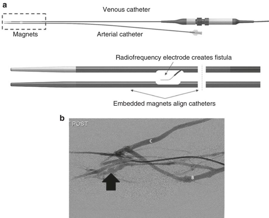
**Fig. 4.13** (a) Schematic of everlinQ device. (b) AVF created using everlinQ between the ulnar vein and ulnar artery (arrow). Injection of contrast from the brachial artery demonstrates flow through the fistula filling the cephalic vein (C) and the basilic vein (B) (From Rajan [114], used with permission)
