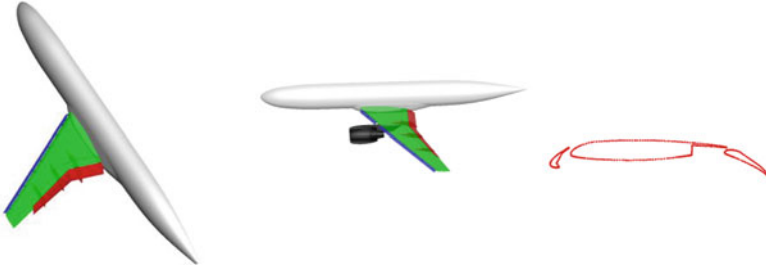
Fig. 1 JSM configuration ( left : configuration without nacelle/pylon assembled; middle : configuration with nacelle/pylon assembled; right : cross section at \eta = 0.43 )
