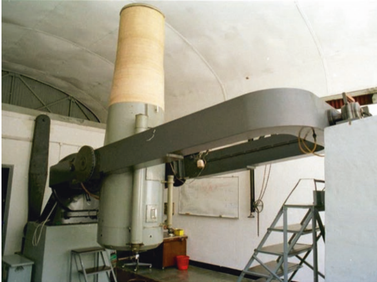
Fig. 14.15 The Bima Sakti Schmidt Telescope. Later the telescope was remounted on a fork mounting ( http://www.oasi.org.uk/Obsvns/19980822_SE/Bosscha_3.jpg )
