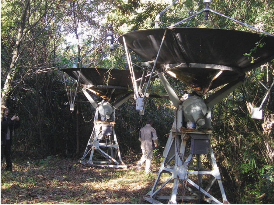
Fig. 6.15 Two of the surviving antennas of a T-shaped array erected in the 1970s, discovered overgrown by dense vegetation just prior to a visit to the Toyokawa Observatory site by the authors of this chapter in November 2010 ( Photograph Wayne Orchiston)
