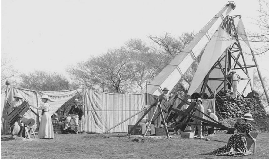
Fig. 26.4 A scene showing the Lick Observatory party ready for the eclipse. All of the instruments are in place and the volunteers are at their practice stations. The 40-ft. Schaeberle Camera with its twin wooden towers dominates the scene ( Courtesy Mary Lea Shane Archives )
