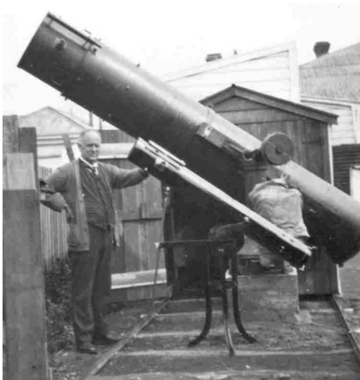
Fig. 20.7 Joseph Ward and his 20.5-in. (52.1-cm) equatorially mounted reflector, along with a 6-in. (15-cm) reflector that he made for sale (Courtesy: Ward (Wanganui) Observatory Archives)
