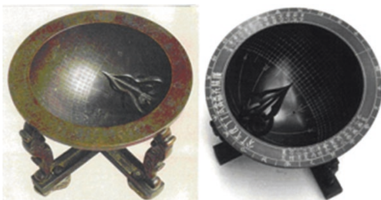
Fig. 7.31 Angbu Ilgui 仰釜日晷, the Scaphe Sundial. The left-hand one is a copy of a late eighteenth century model, and the right-hand one is a recent copy of another model (after Nha 2004b)
