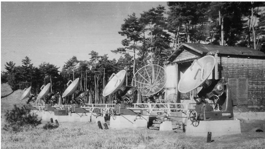
Fig. 6.10 A view of the 4000 MHz five-element grating interferometer installed at Toyokawa in 1953 ( Courtesy Tanaka Family )
