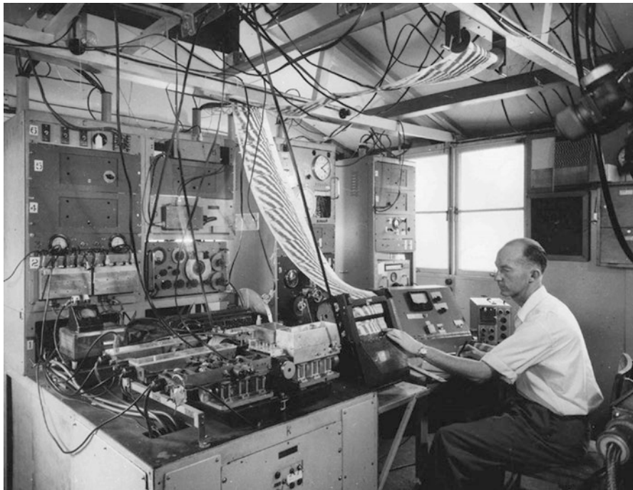
Fig. 19.67 Kevin Sheridan and the position interferometer receiver and facsimile record ( Courtesy Sullivan, Dapto 02 )
