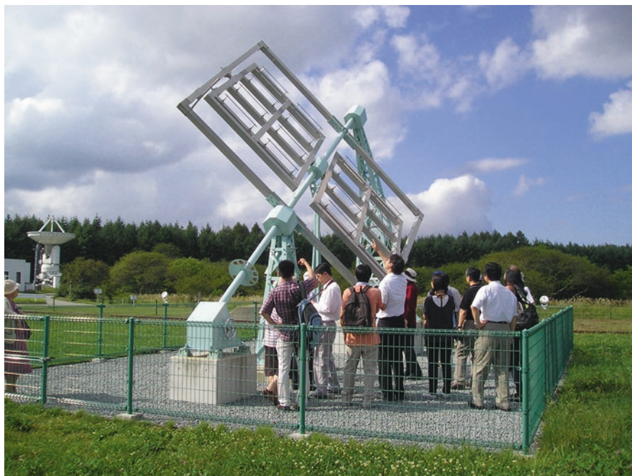
Fig. 6.14 A replica of the original TAO broadside array on display at the Nobeyama Radio Observatory; only the polar axis is from the original radio telescope of 1949 ( Photograph Wayne Orchiston )
