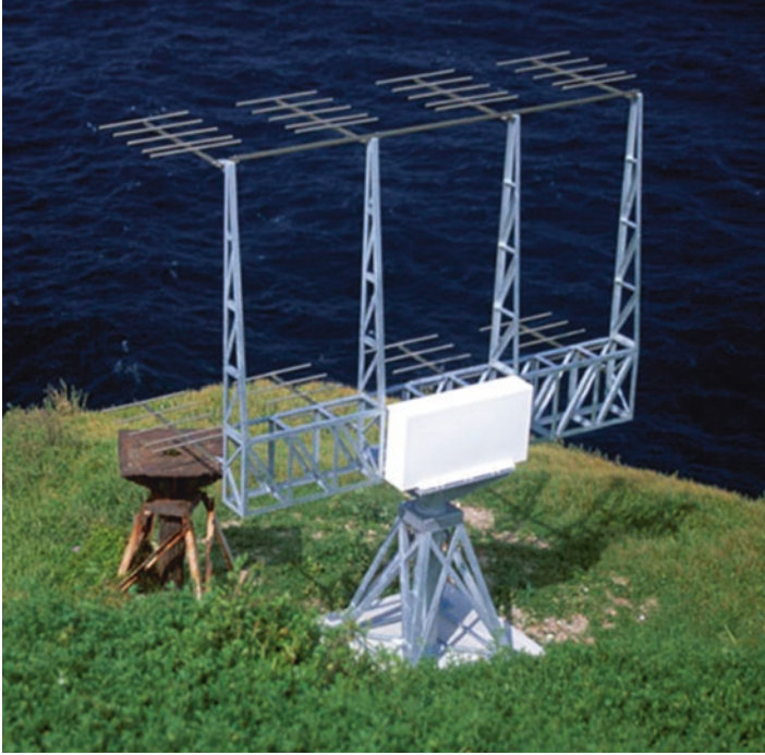
Fig. 19.94 The replica 8-Yagi antenna at the site of the Dover Heights field station in 2003, beside its original rusting mount ( Photograph Wayne Orchiston)
