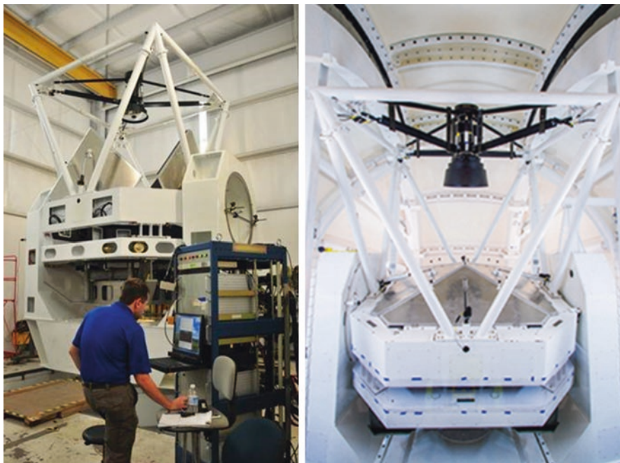
Fig. 11.14 Two views of the automated 2.4-m Richey-Crétien Thai National Telescope. Left: undergoing testing prior to its installation at the TNO; right: installed and operational at the TNO (Courtesy NARIT)
