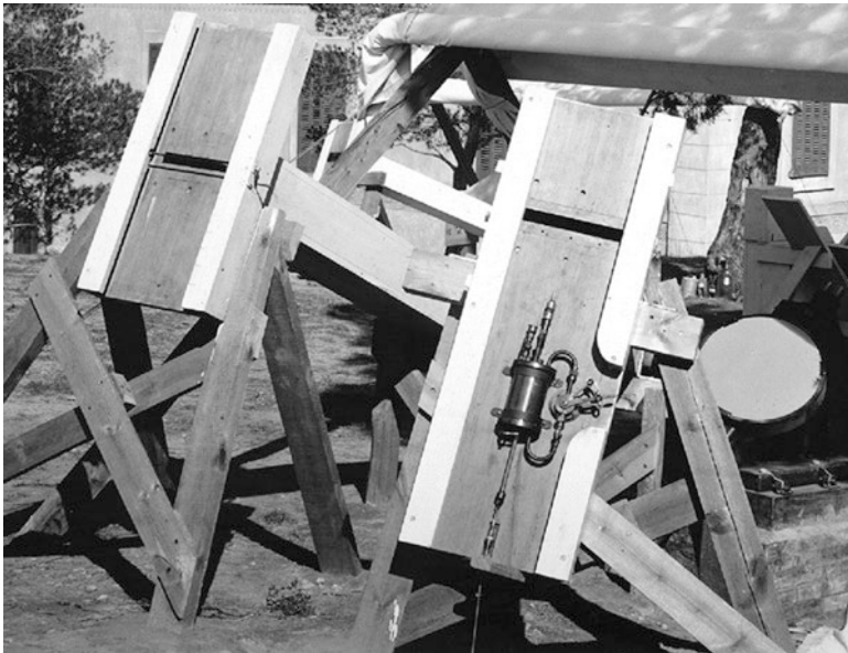
Fig. 26.5 Campbell's moving plate spectrographs as they appeared in 1905, showing one of the gas-driven pistons that moved the plate-holder in order to obtain a continuous recording of the coronal spectrum throughout totality ( Courtesy Mary Lea Shane Archives )
