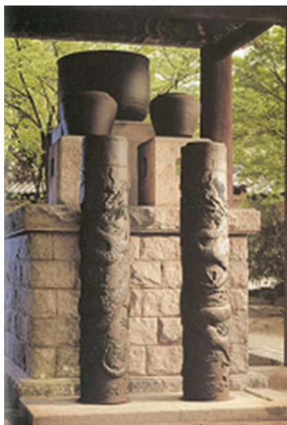
Fig. 7.33 A recent restoration of King Sejong's Jagyok-nu , Automatic Striking Clepsydra, carried out by Nam and his collaborators (after Nam 2006)
