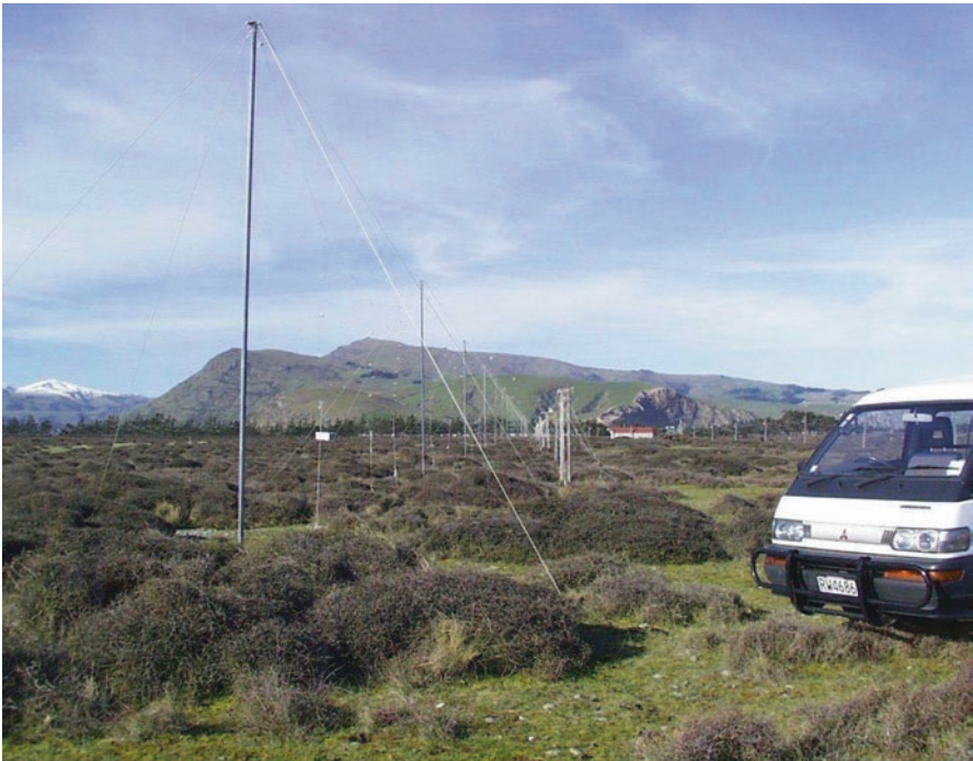
Fig. 20.30 The University of Canterbury's AMOR radar transmitting antenna sampling in the north-south meridian. The radar facility was at Birdlings Flat, on the spit between Lake Ellesmere and the Pacific Ocean southeast of Christchurch, and was used to detect micrometeoroids in the upper atmosphere from radar echoes from their ionization trails ( Courtesy Jack Baggaley )
