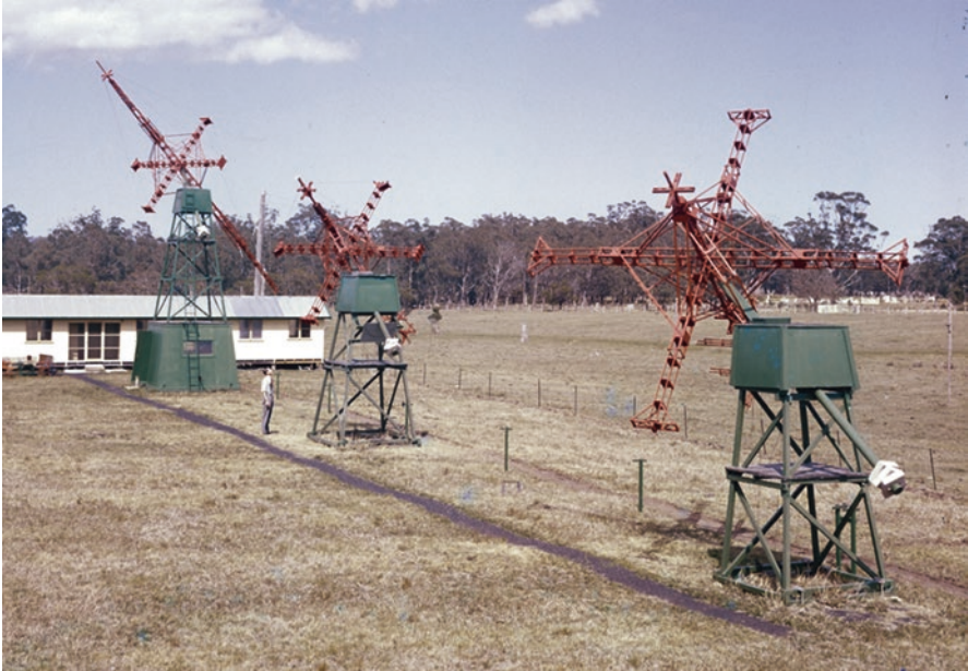
Fig. 19.63 The Dapto field station, showing the three crossed-rhombic antennas and associated buildings ( Courtesy CSIRO RAI 12429-1 )
