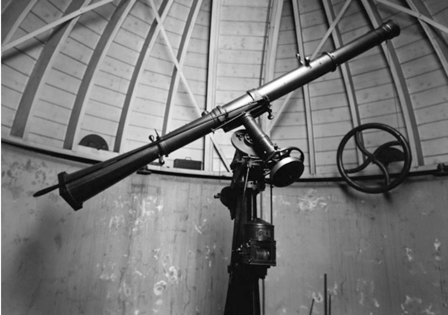
Fig. 17.19 The 4-in. Dallmeyer photoheliograph in 1875 (Clark collection)
