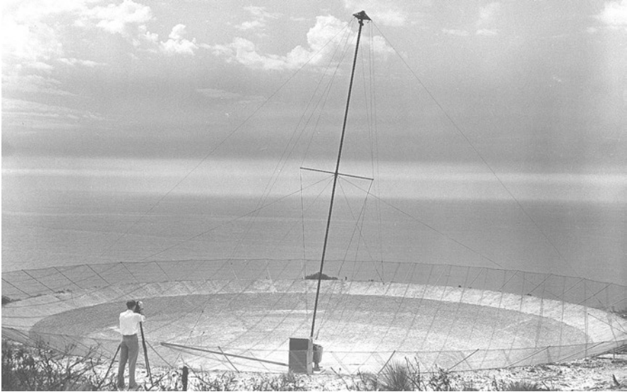
Fig. 19.15 The 24.4 m (80-ft.) hole-in-the-ground radio telescope; Gordon Stanley is using a theodolite to record the angle of tilt of the aerial mast (Courtesy CSIRO RAIA B3150-7)
