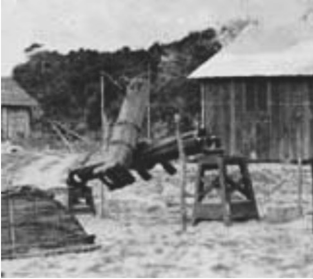
Fig. 12.11 An enlargement of the 20-cm reflector made especially by Adophe Martin for the Siam solar eclipse expedition and shown in Fig. 12.13. Note the crude wooden tube, even cruder equatorial mounting and primitive wooden mirror support ( Courtesy Archives, Observatoire de Marseille, 132 J 84 )
