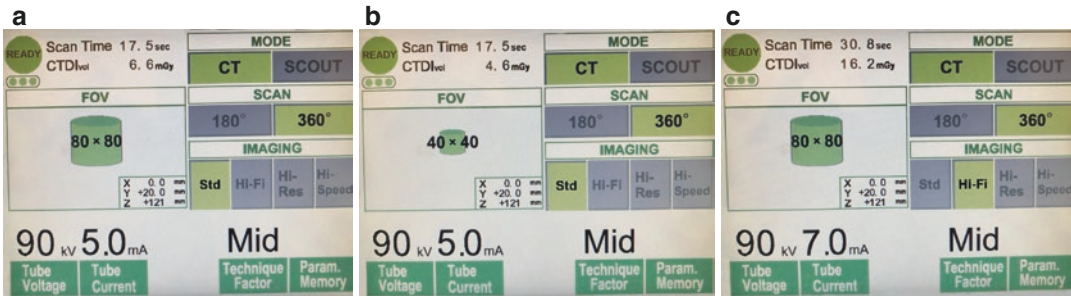
Fig. 5.3 Screen shot of exposure panel for a CBCT device (Accutitomo 170, J. Morita, Kyoto, Japan) that has default exposure settings based on number of basis projection images. Manufacturer default exposure settings for a 360° standard (Std), 80 mm × 80 mm scan (HD) (a)
