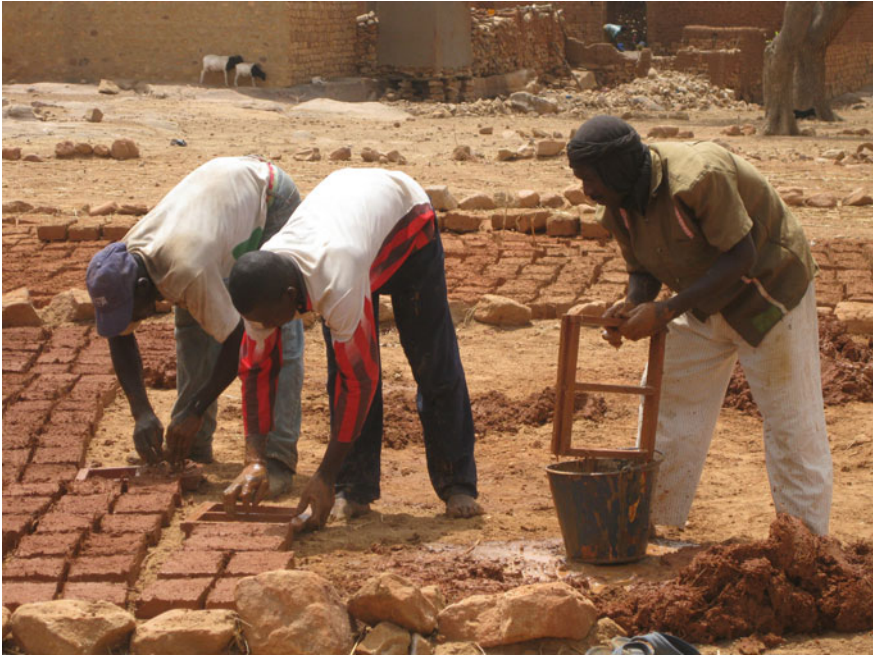
Fig. 3 Mud bricks production. Photo credits: All pictures are made by caravatti_caravatti architetti
