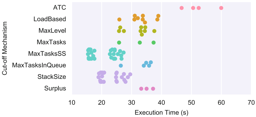
Fig. 9. Swarm plot of different cut-off approaches for the KDTree training program on the astrid machine.
