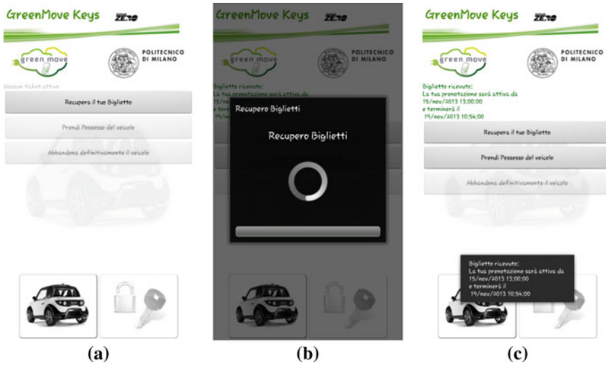
Fig. 6 Retrieval of the virtual key through the user’s mobile device: a users ask to retrieve the virtual key (“recupera il tuo biglietto” = “retrieve your ticket”); b the Green Move app on the mobile device contacts the GMC to retrieve the requested information (“recupero biglietti” = “ticket retrieval”); c the virtual key is successfully retrieved (“biglietto ricevuto” = “ticket received”)
