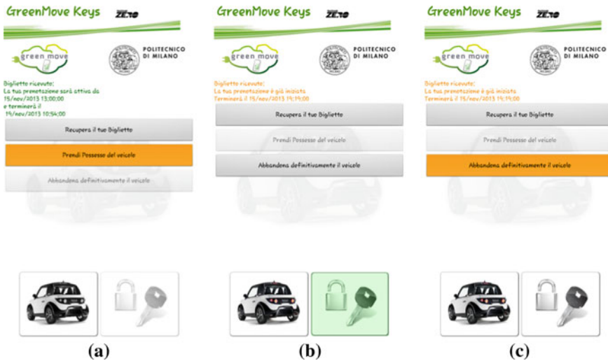
Fig. 7 Use of the virtual key to: a take charge of the vehicle (“prendi possesso del veicolo” = “take hold of the vehicle”); b lock/unlock the vehicle (through the key icon); c release the vehicle (“abbandona definitivamente il veicolo” = “release the vehicle for good”)
