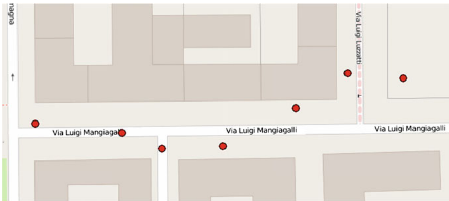
Fig. 7 Circles indicate the measured coordinates of a car test every five seconds
