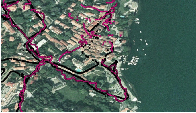
Fig. 5. Details of two different acquisitions with a geodetic device – Leica GPS 1200 receiver (black route) and a low cost GNSS receiver - Nexus 6P (purple route). (Color figure online)
