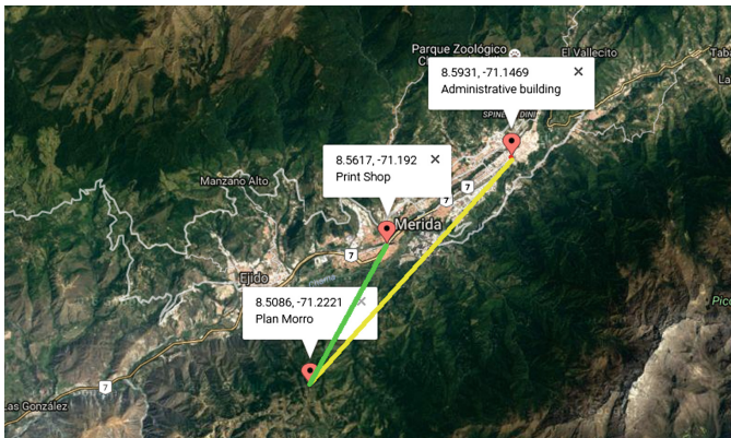
Fig. 6. Layout of the two legs link from administrative building to the printshop, Merida Venezuela.
