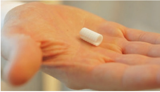
Fig. 9.17 A patient-matched, 3D printed tracheal splint was developed by the University of Michigan to treat young children with a rare condition called tracheobronchomalacia (TBM), a collapse of the airway. The splint is designed from the patient's CT scan of the airway using Materialise Mimics software and 3D printed out of a bio-resorbable material. Courtesy Materialise USA, Plymouth, Michigan, USA and University of Michigan, Ann Arbor, Michigan, USA
