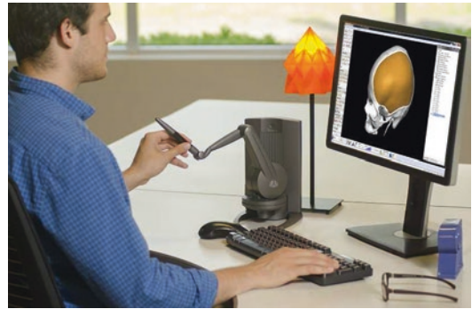
Fig. 9.4 An engineer uses Geomagic Freeform software to design a patient-matched cranioplasty. The tool in his left hand provides force feedback, giving the designer the sensation of “touching” the design he is working on. Courtesy 3D Systems, Rock Hill, South Carolina, USA
