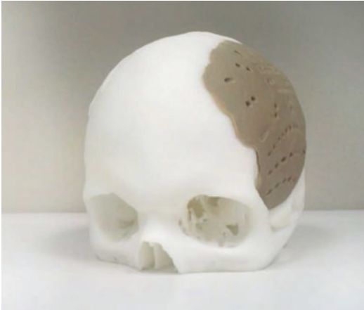
Fig. 9.10 Cranioplasty implant 3D printed in PEKK biomaterial for a patient with a large cranial defect. Courtesy Oxford Performance Materials, South Windsor, Connecticut, USA
